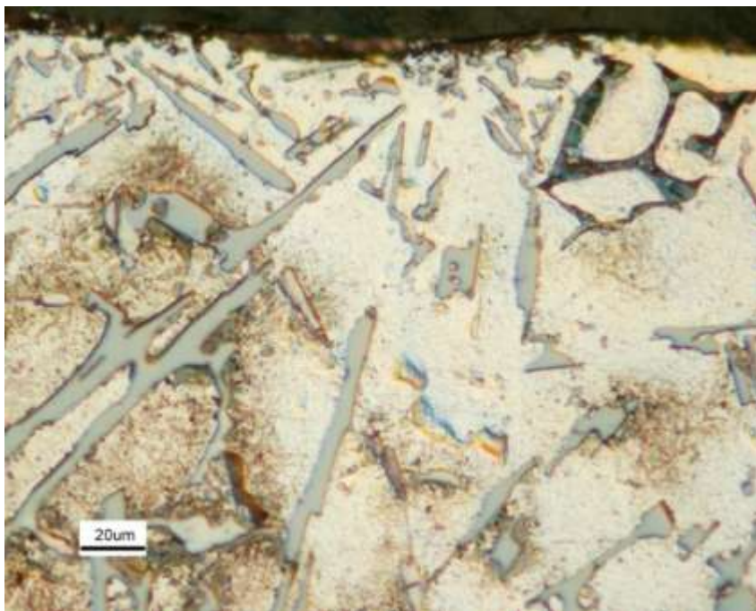
Figure 31: High magnification micrograph of an MMM sample after melting revealing the microstructure at the top surface
