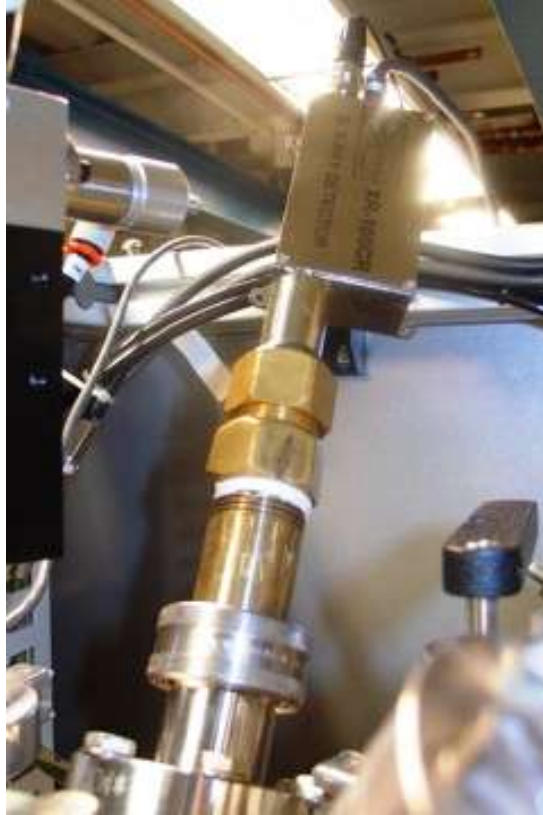
Figure 5: View of the brass detector sleeve inserted into the bench-top unit via a vacuum compression fitting.
