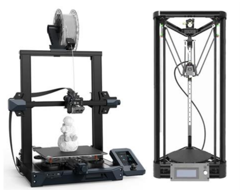
Figure 2 - Comparison of Cartesian and Linear Delta Printers
