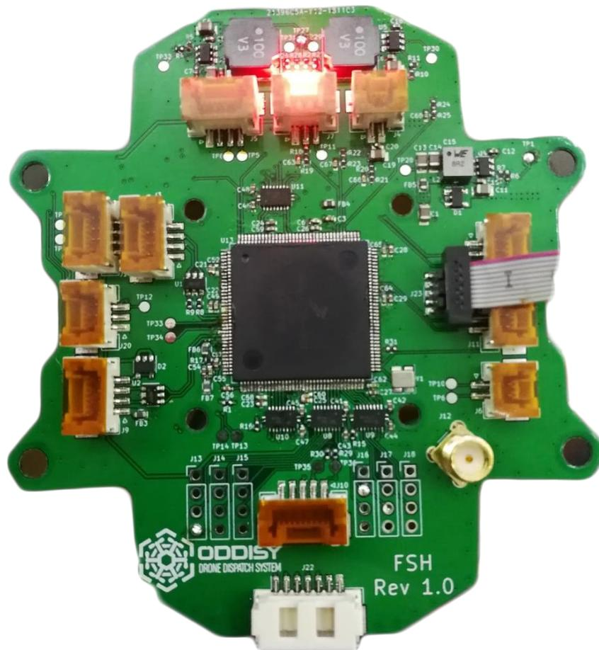
Figure 2: Top view of fully assembled FSH
