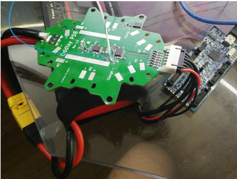
*Figure 6: PDB Connected to 6 Cell Lithium Polymer Battery*
