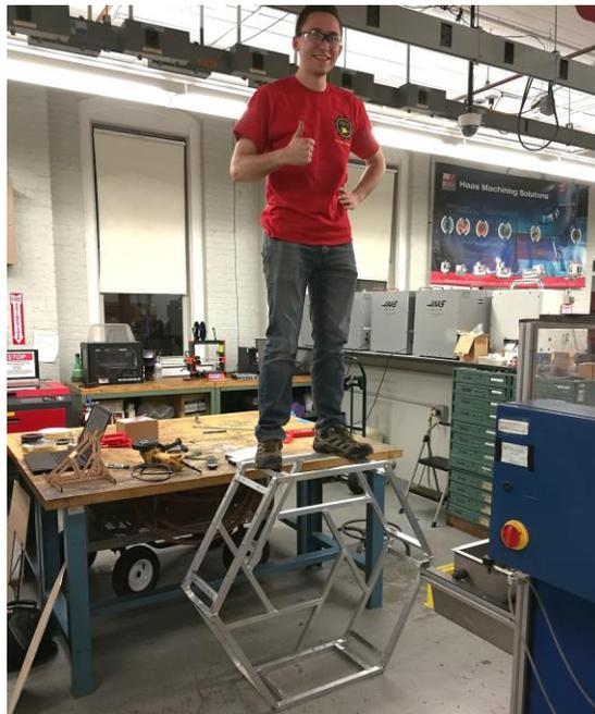
*Figure 12: Aluminum Frame Supporting ~170lbs*
