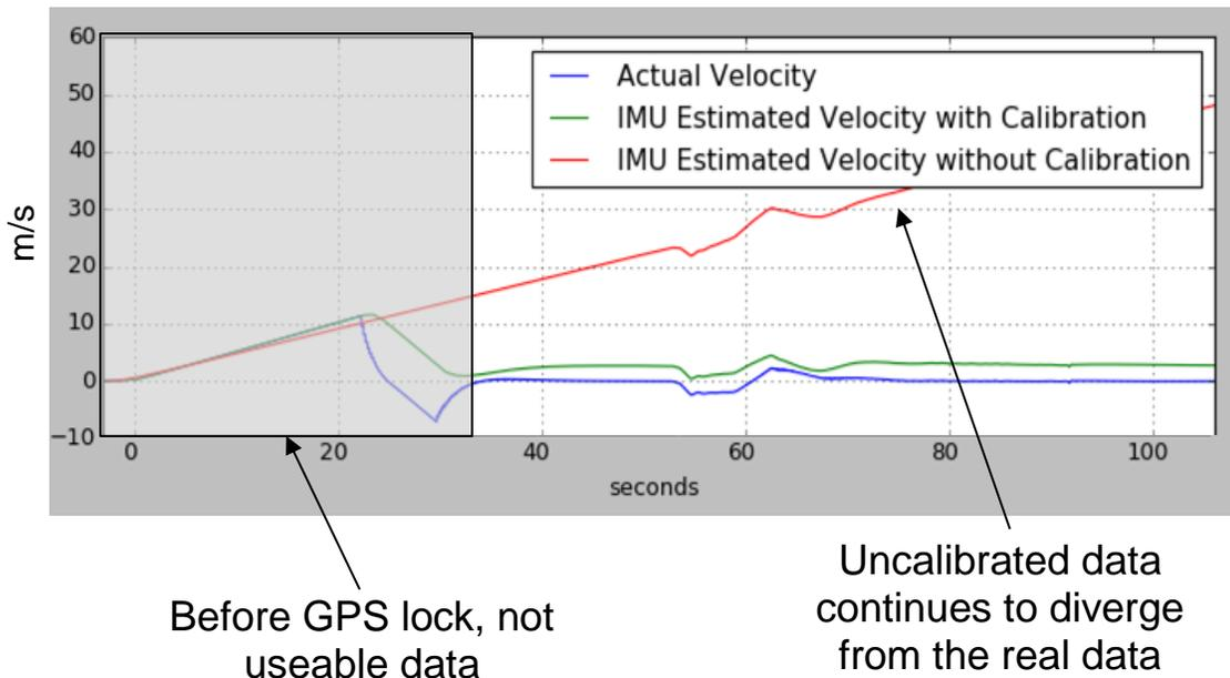
Figure 18: Graph of Predicted Velocity Showing IMU Calibration
