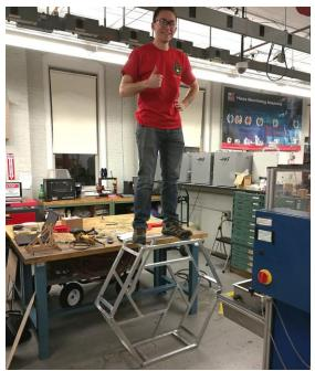
Figure 12: Aluminum Frame Supporting ~170lbs
