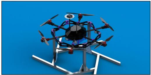
Figure 14: Render of Base Station Landing Ring
