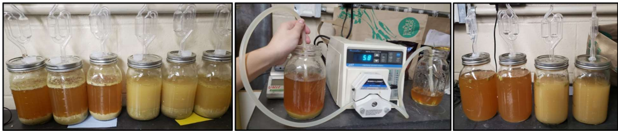
Figure 7: The dry hopping process for the NEIPA's control and well-mixed brews. After 8 days of fermentation, the beer is moved to a secondary fermenter and a specific amount of mosaic and citra hops are added to the beer.
