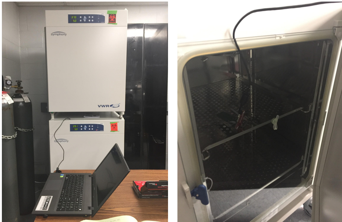
Figure 31: Setup for Temperature Sensor Test Using VWR Symphony CO2 Incubator
