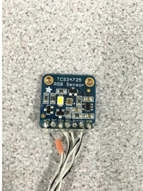
Fig. 6.3 TCS34725 RGB color sensor with white LED.
