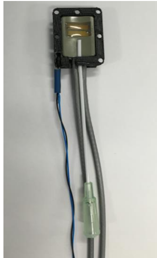
Fig. 6.2 Combination probe holder with flat Doppler probe, thermistor, and ultrasound gel catheter fixed in place.
