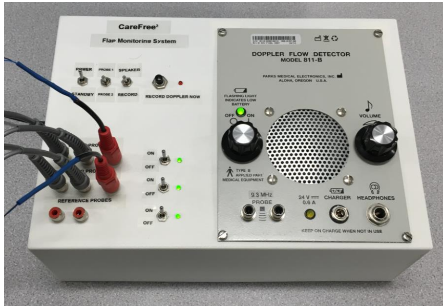
Fig. 5.6 Final bedside device with integrated Doppler flow meter and components.
