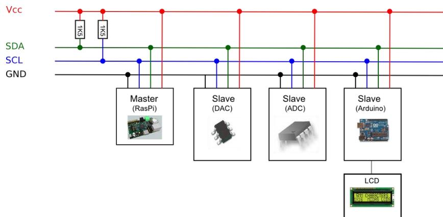
Figure 18: Example of a circuit using I2C (I2C and SPI, n.d.)
