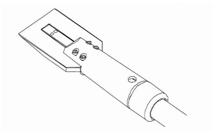
*Figure 16: Wedge tip of a ground penetrating probe (Michel U. Louge, 1998)*
