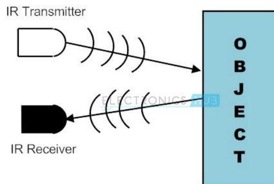
Figure 9: Infrared sensor system (Electronics Hub, 2015)
