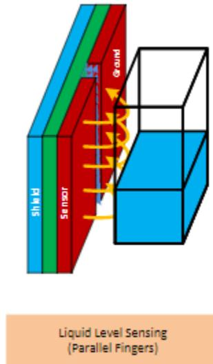
Figure 7: Parallel Finger configuration for capacitive sensors (Texas Instruments Incorporated, 2014)
