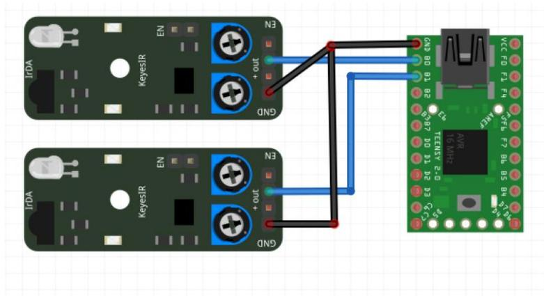
Figure 27: Circuit Layout for Sensor Module
