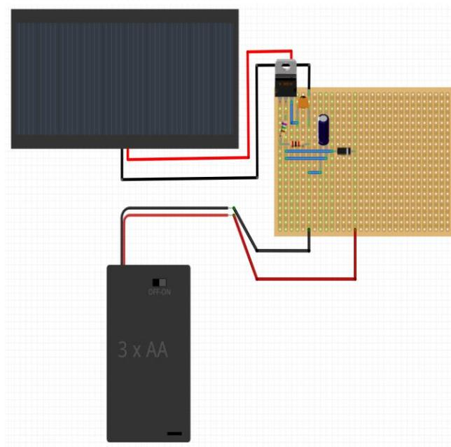
Figure 29: Circuit Layout for Power Circuit
