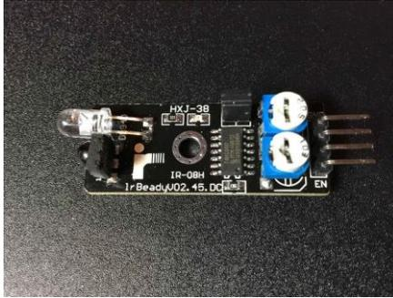
*Figure 12: IR Infrared Obstacle Avoidance Sensor sold by Resistor Park (IR Infrared Obstacle Avoidance Sensor, 2016)*
