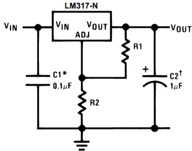
Figure 24: LM317 Voltage Regulator Circuit (Texas Instruments, 2015)
