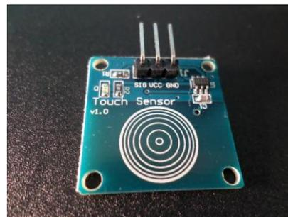
Figure 11: Arduino Capacitive Touch Sensor sold by Resistor Park (Arduino Capacitive Touch Sensor, 2016)
