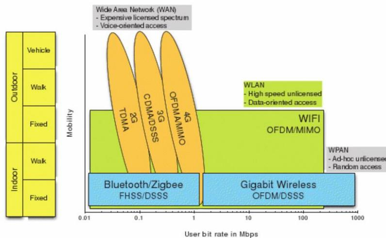
Figure 20: Various communication protocols compared by mobility and bit rate (Pahlavan & Krishnamurthy, 2013)
