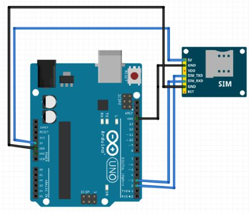
Figure 28: Circuit Layout for Head Module
