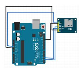
Figure 28: Circuit Layout for Head Module
