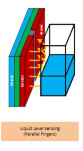
Figure 7: Parallel Finger configuration for capacitive sensors (Texas Instruments Incorporated, 2014)
