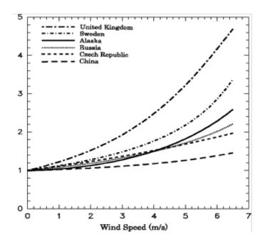
Figure 6: Relationship between solid precipitation adjustment factor (K) and wind speed at gage height (m/s) (Legates & DeLiberty, 1993)
