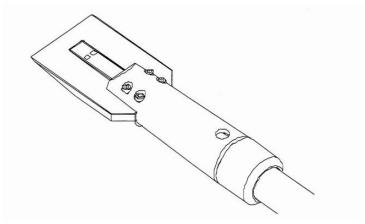
Figure 16: Wedge tip of a ground penetrating probe (Michel U. Louge, 1998)
