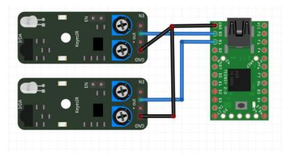
Figure 27: Circuit Layout for Sensor Module
