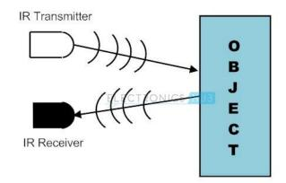
Figure 9: Infrared sensor system (Electronics Hub, 2015)
