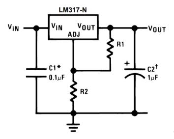
Figure 24: LM317 Voltage Regulator Circuit (Texas Instruments, 2015)
