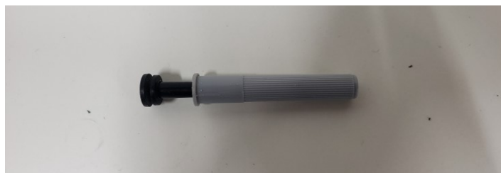
Figure 5.1: One of the stock air spring modules retrieved from the broken landing gear.
