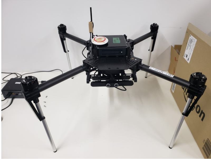
Figure 5.5: One of the M100 drones fitted with the aluminum legs.
