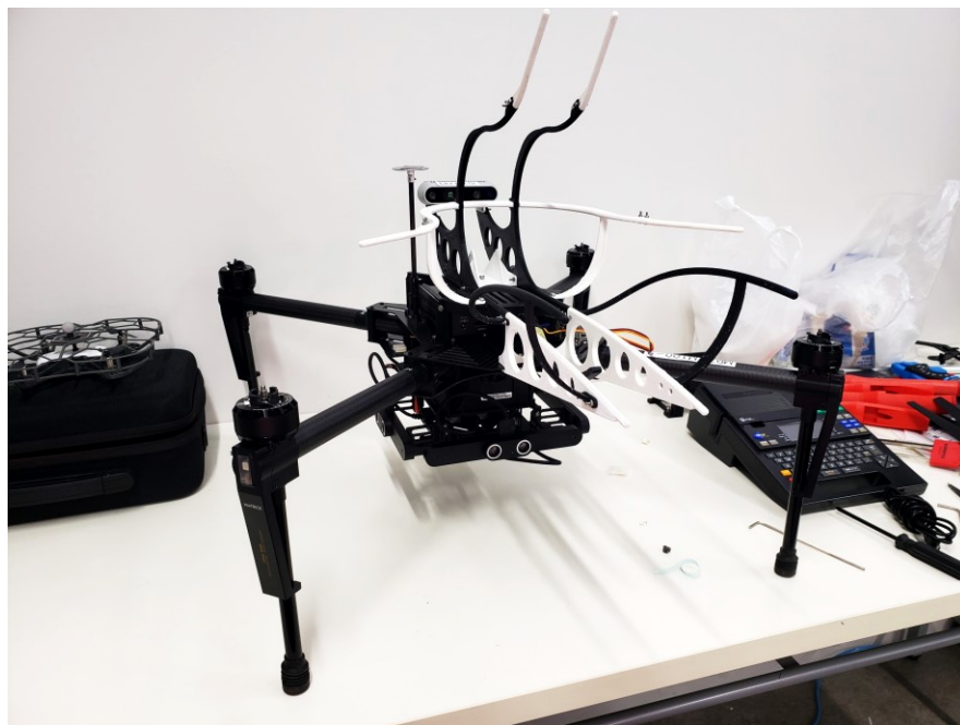
Figure 5.20: One of the M100s fitted with the full capture assembly.
