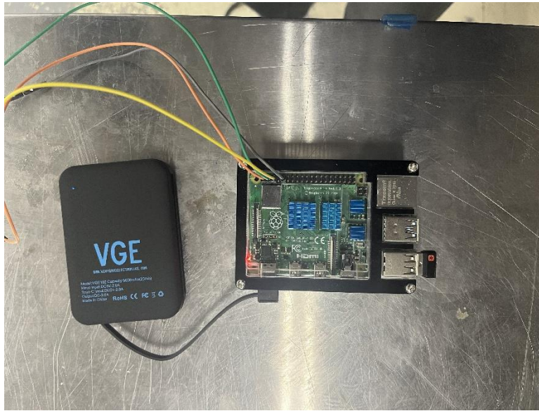
Figure 53: Small battery used to power the Pi and motor control boards on the prototype rover
