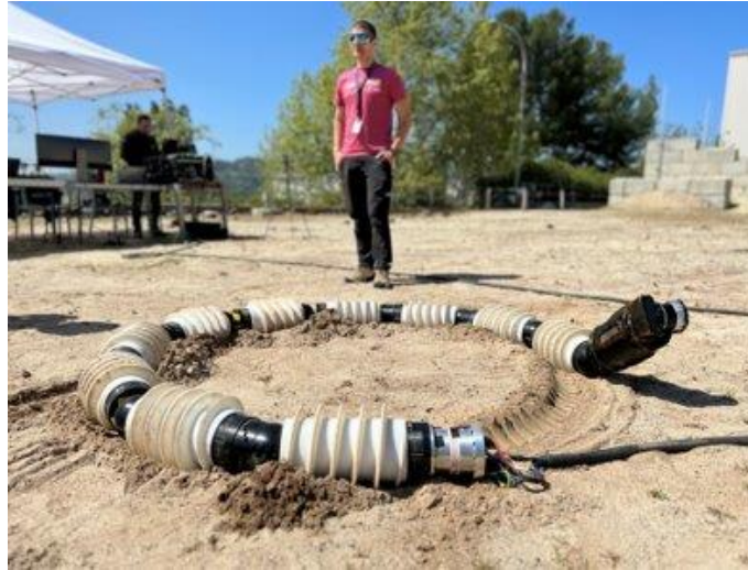
Figure 9: Example of a slithering rover with segments that expand and contract (NASA, 2022). © 2024 Northeastern University
