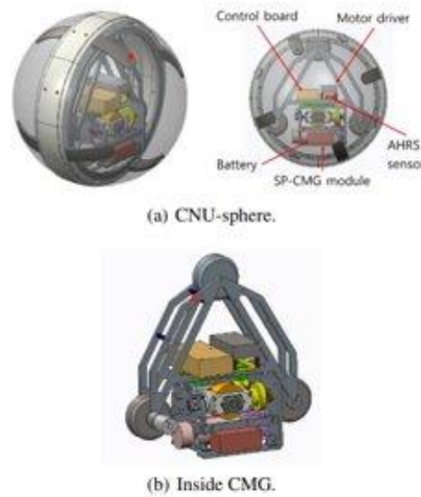
Figure 11: Inner workings of a gyroscopically propelled spherical rover (Kim Et al., 2020). © 2020 Springer
