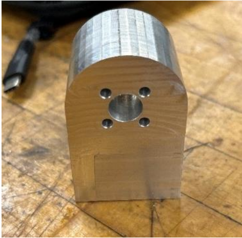
Figure 89: Single shoulder mount with two operations remaining
