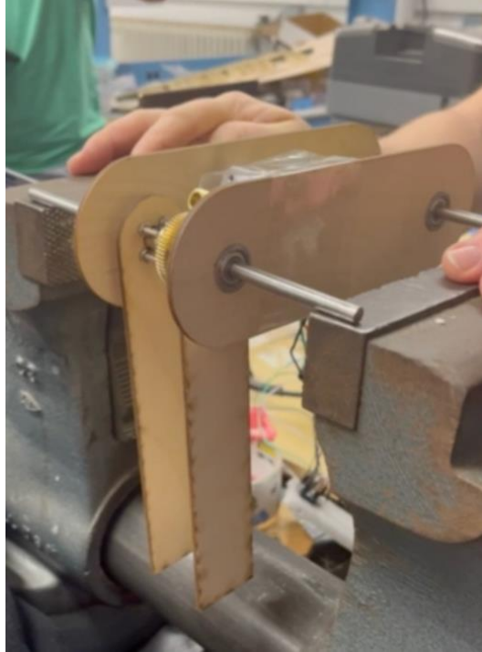
Figure 80: Image of the test leg made from laser cut plywood
