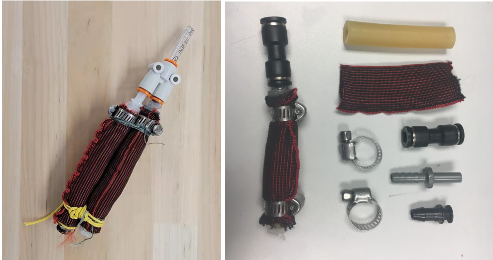
Figures 13 and 14: A Hydro Muscle (left), and all of its components (right) (Clarrissimeaux, 2021).
