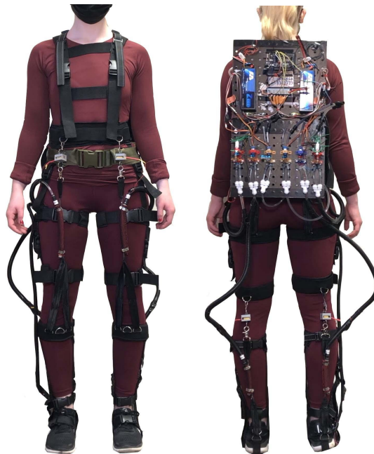
Figures 9 and 10: A front and back view of the previous iteration of the Bioinspired Exosuit (Clarrissimeaux, 2021).
