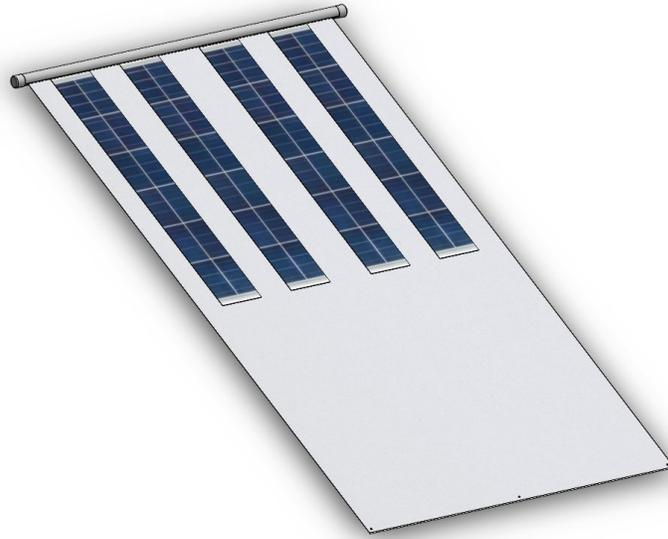
Figure 22: SolidWorks Model of SolFly Design with Four Solar Panels
