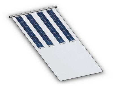
Figure 22: SolidWorks Model of SolFly Design with Four Solar Panels
