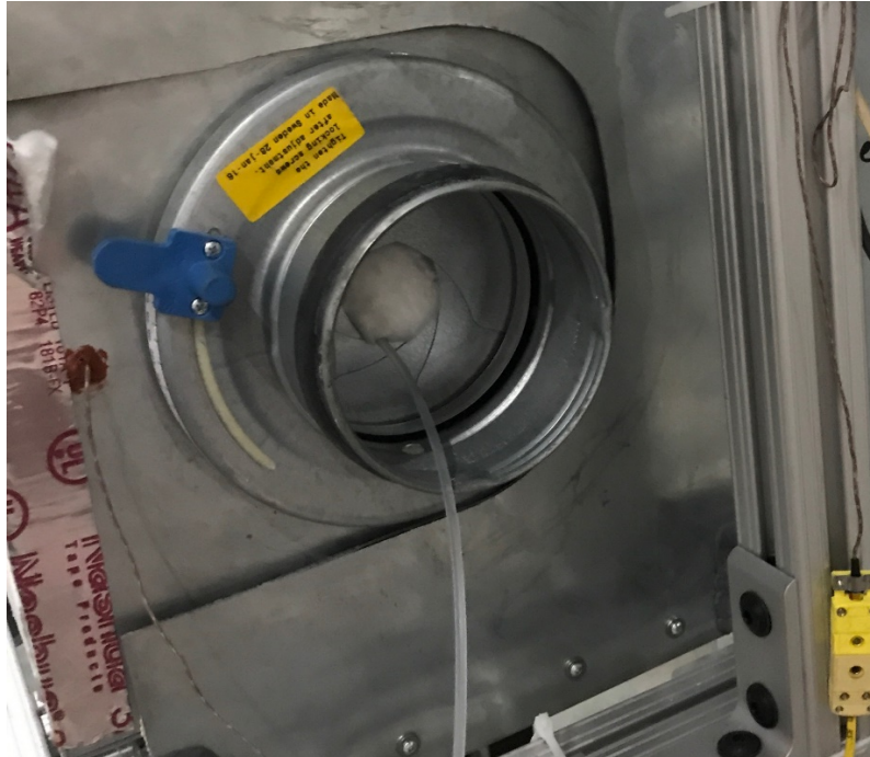
Figure 13: View of the Iris Damper on the Testing Apparatus
