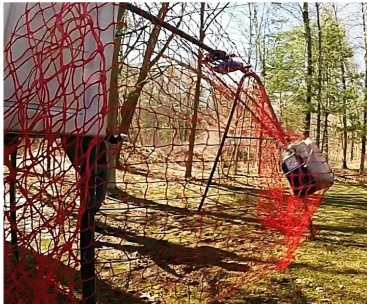
**Figure 15: Maximum net stretch when hung loosely**
