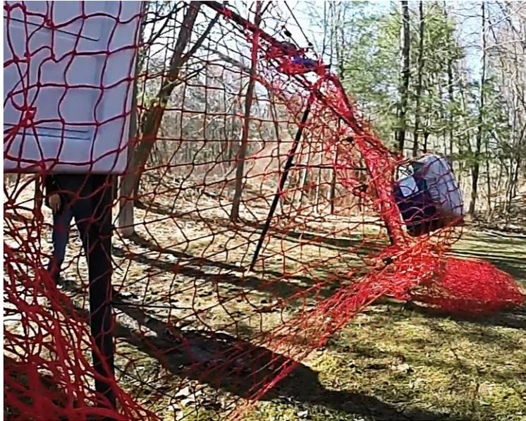
Figure 16: Maximum net stretch with modified B-net
