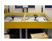
Sand Pendulum: a hanging funnel for sand to flow through, and create designs on a surface below
