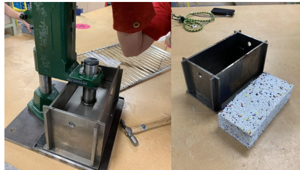
Figure 15: Compact Plastic Brick Production - The machine above can be used in remote areas to create plastic bricks with little manpower or electricity [36]
