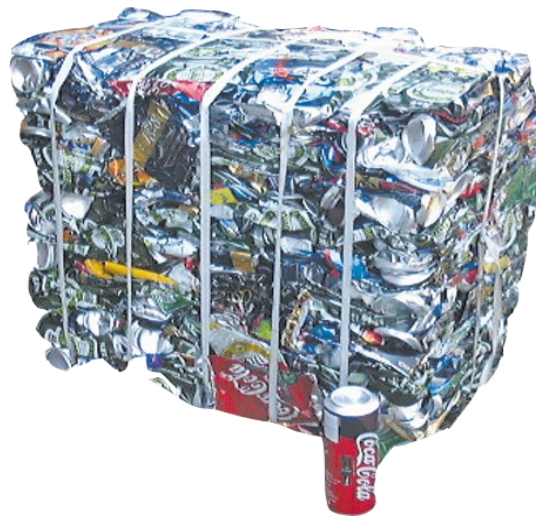
Figure 18: Aluminum cans compacted with a baler machine. [43]
