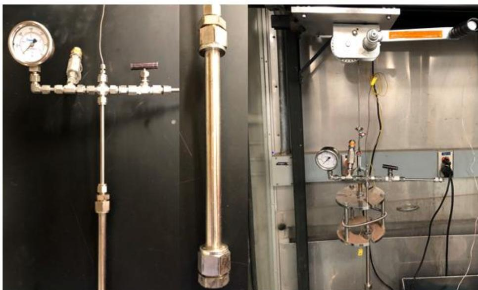
*Figure 14* Key parts of tube hydrolysis reactors: pressure gauge, reactor body and the stainless-steel disc-shaped holder.
