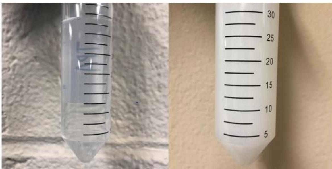
*Figure 15* Appearance of solutions while recovering TPA: solution after adding sodium hydroxide (left), and solution after adding hydrochloric acid (right).
