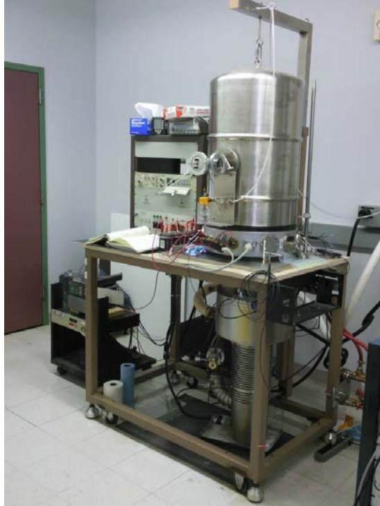
Figure 10: WPI Vacuum Facility Hoist System
