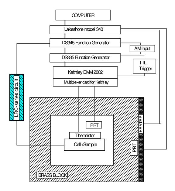
Figure 3.9: Block diagram of the electronics for the Radio Frequency Calorimeter.
