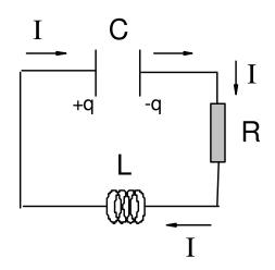
Figure 2.8: An LCR series circuit.
