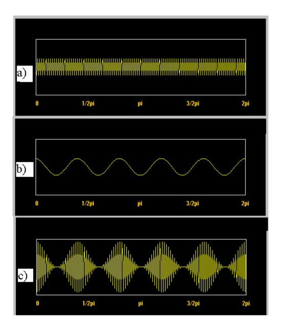
Figure 4.2: a) Schematics of the carrier wave high frequency alternating electric field used in radio frequency calorimeter; b) Schematics of the am modulation waveform used to modulate the high frequency alternating electric field. c) Schematics of the final modulated high frequency alternating electric field used in radio frequency calorimeter.
