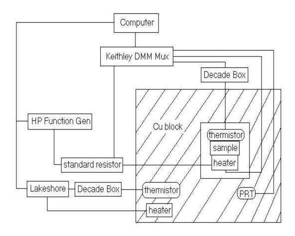
Figure 3.4: A block diagram of the AC Calorimeter design.
