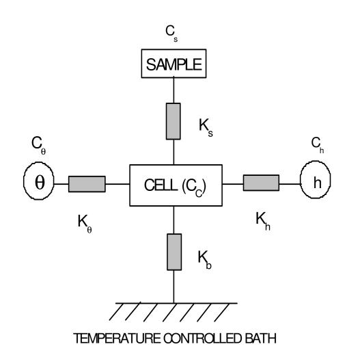
Figure 3.1: One lump thermal model used in an AC calorimetry.
