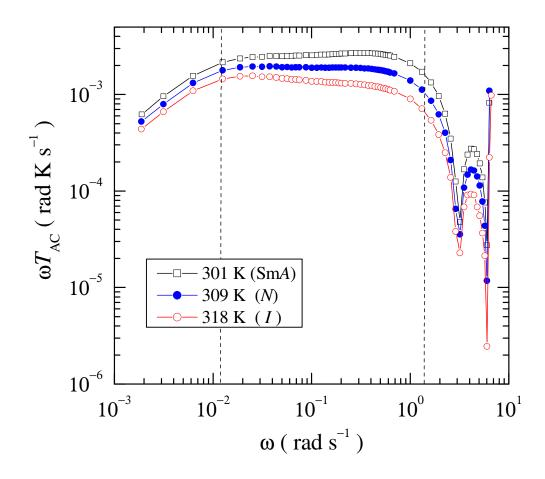
Figure 4.4: Typical frequency scans for 8CB+aerosil sample at 0.1 g/cm<sup>3</sup> silica density taken by the RF/AC calorimeter at three different temperatures corresponding to the isotropic (I), nematic (N), and Smectic-A (SmA) phases.
