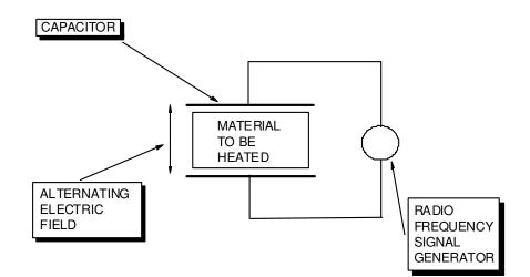
Figure 2.5: Simple Radio Frequency applicator.
