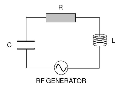
Figure 3.6: LRC series circuit used as radio frequency heating matching network.
