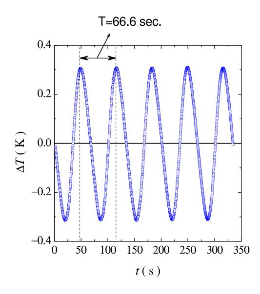
Figure 4.3: Sample temperature oscillations achieved by modulating the amplitude of the base frequency voltage at  $f_{\rm rf} = 0.805$  MHz, with an AM modulating frequency  $f_{\rm am} = 15$  mHz.
