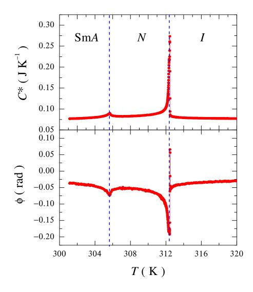
Figure 4.6: Typical temperature scan data taken with an AC calorimeter using a Joule heating method. The upper panel shows temperature dependence of the heat capacity from temperature, the lower panel shows temperature dependence of the phase shift.
