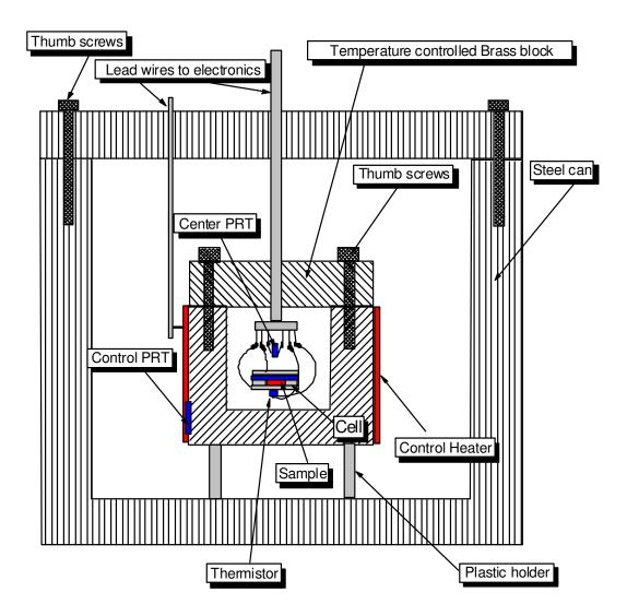
Figure 3.8: Design of Radio Frequency Calorimeter.
