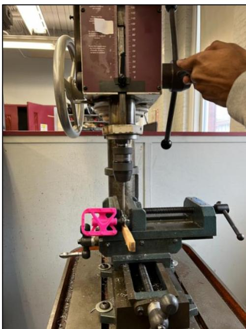
*Figure 57. Setup for drilling pedal crank holes.*
