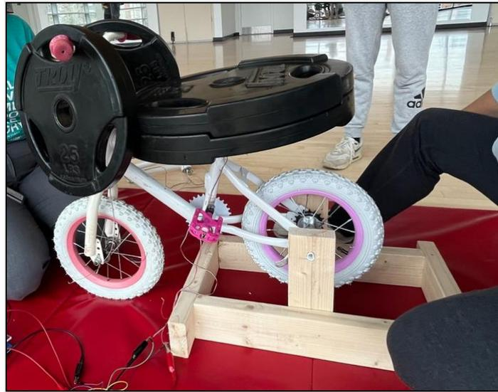
Figure 39. Loading setup of bicycle for mechanical testing.
