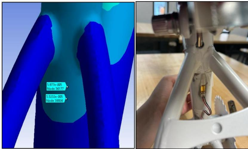
Figure 46. Strain gauge location 6 (without top bar).
