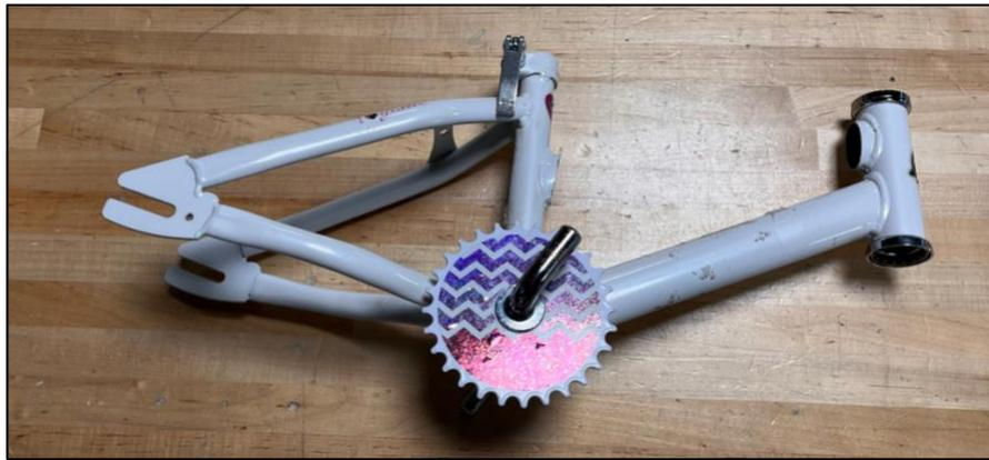
*Figure 56. Bicycle frame after the top bar was removed.*
