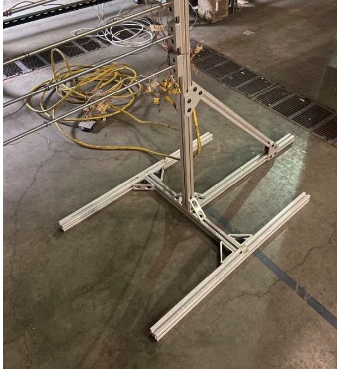
Figure A.2. Thermocouple tree base.
