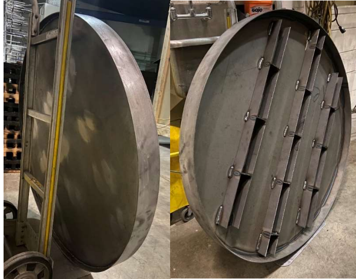
Figure 17. New carbon-steel, 1 meter fuel tray. Shown are the front and back sides of the tray respectively.
