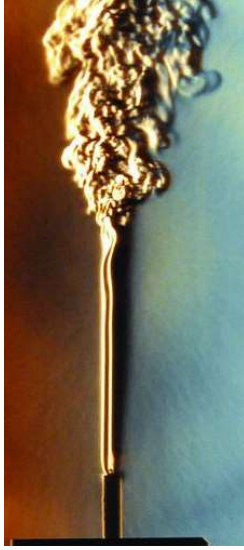
Figure 1. Fire plume of a candle visualized using Schlieren imaging. [1]
