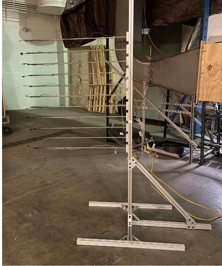
Figure A.1. Thermocouple tree assembly.
