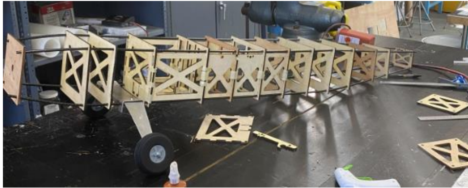
Figure 11: Early Bulkhead Design
