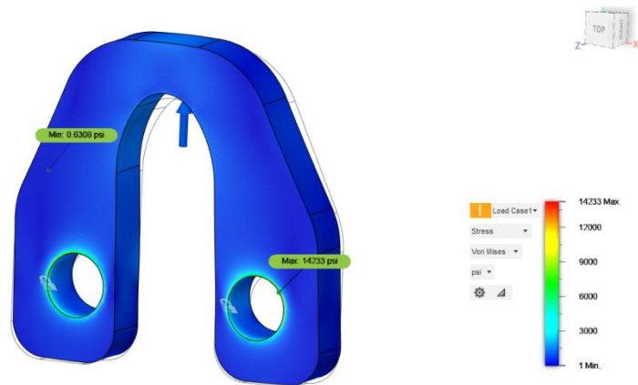
Figure 47: Fusion360 Deformation and Stress Analysis of Wing Locking Bracket
