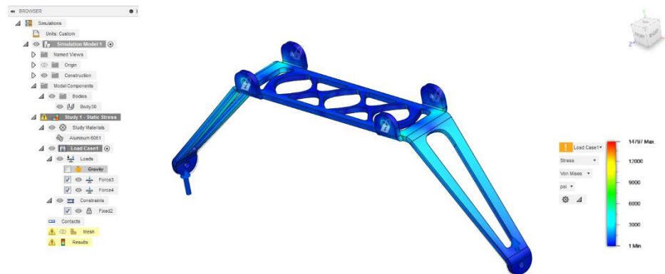
Figure 45: Fusion360 Deformation and Stress Analysis of Aluminum Bracket
