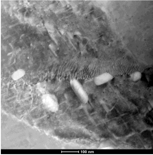
Figure 40: HAADF of 25 Hour Aged-6061 performed by PSU Applied Research Laboratory
