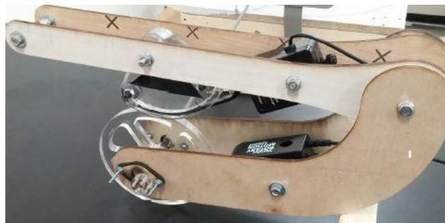
**Figure 29:** Dynamometer from first MQP team
