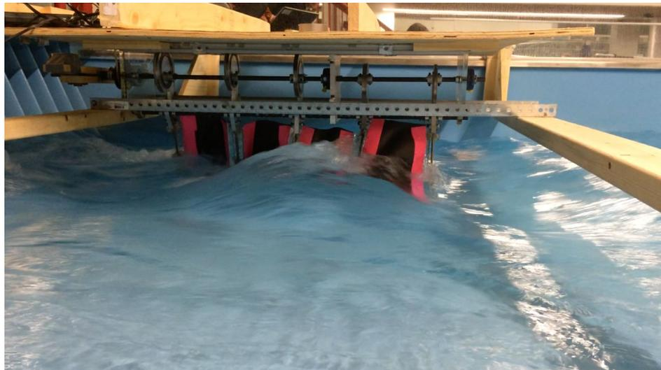
**Figure 52:** Standing wave in flow tank (1200 speed)
