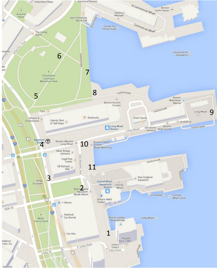
Figure 21: Surveying route for the Christopher Columbus Park, with key showing measurements and error of closure. ( Google Maps )
