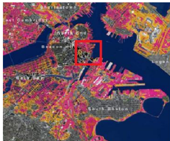
Figure 4: Flooding at today's high tide plus 7.5 ft (TBHA, 2013)
