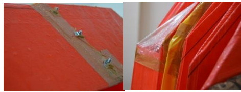
Figure 22: Water testing of shelter prototype. Water beading is visible
