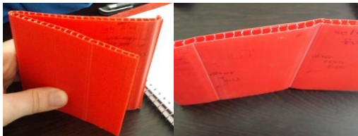
Figure 20: Folding fatigue resistance results
