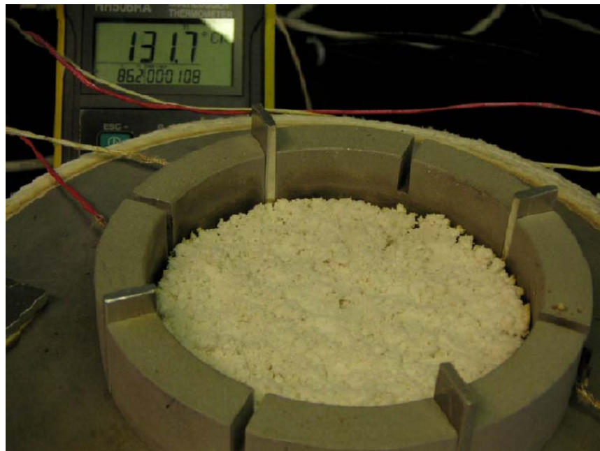
Figure 52 : Gum powder (20g) with ketone-based liquid solution(1g) at 270 °C, early stage
