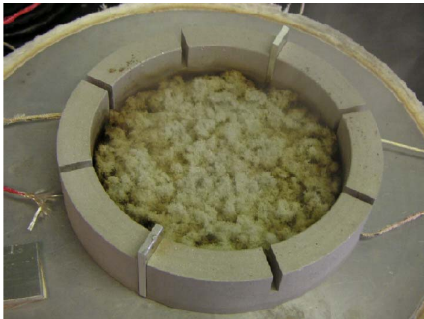
Figure 37 : Paper dust (3g) with DTE24 (3g) at 400 °C, early stage
