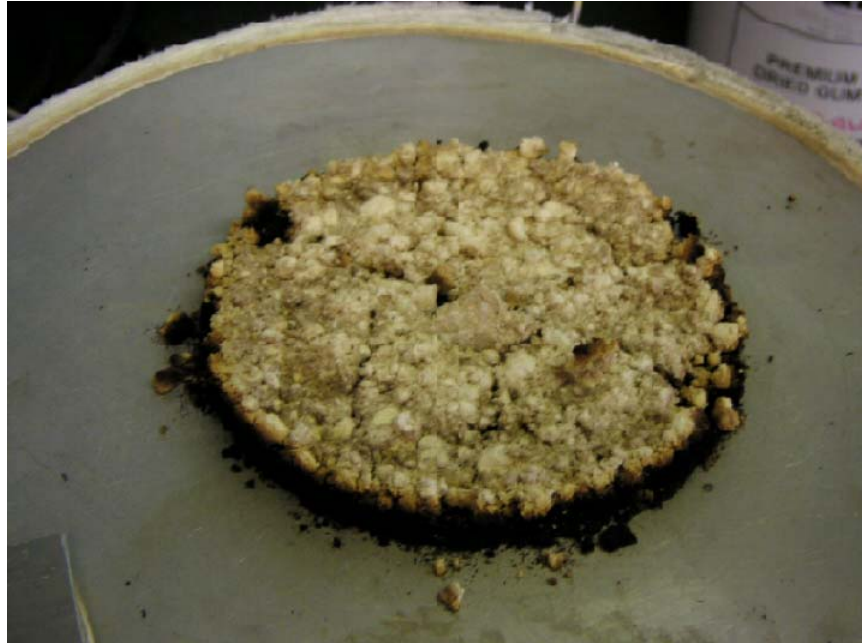
Figure 53 : Gum powder (20g) with ketone-based liquid solution (1g) at 270°C, at the end of test
