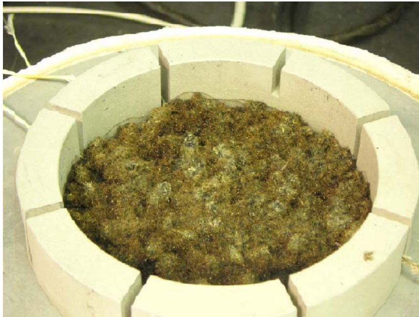
Figure 41 : Paper dust (3g) with newspaper printing ink (3g) at 350°C, at the end of test
