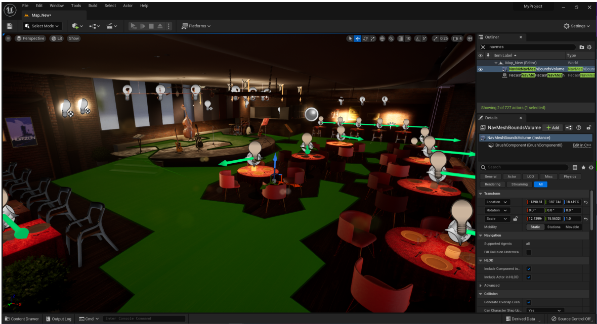
Figure 24: The navigation mesh used for teleportation (a similar mesh exists in the other map)
