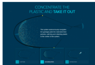
Figure 6: This diagram showcases how the System 001/B works while in the ocean. The three steps are capture, accumulation, and extraction. Photograph by The Ocean Cleanup, Terms of Use .
