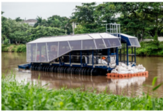
Figure 5: This is the Interceptor made by the Ocean Cleanup which collects the trash in rivers through the currents. " Interceptor 001, first generation, in Jakarta, Indonesia ", by The Ocean Cleanup, Terms of Use .
