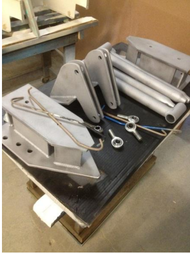
Figure 50 - Parts After Sandblasting
