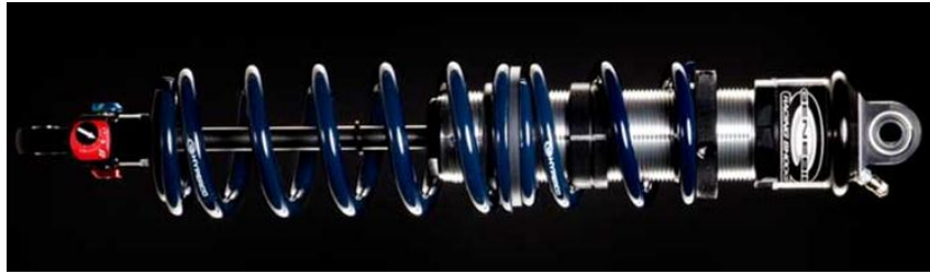
Figure 6 - Variable spring rate (stacked springs example) ( genesishocks.com )
