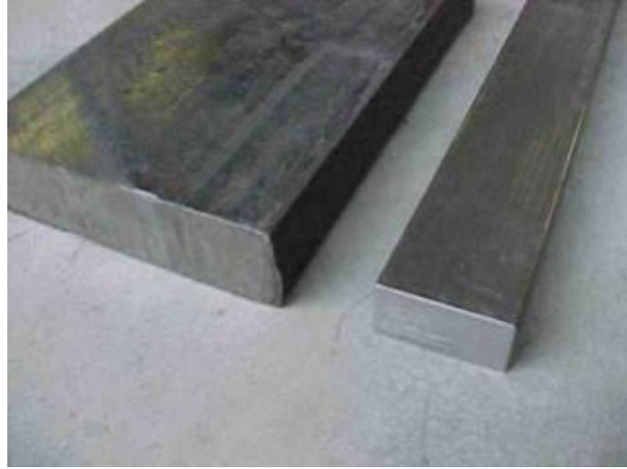
Figure 51 - Hot Rolled Steel on Left, Cold Rolled Steel on Right
