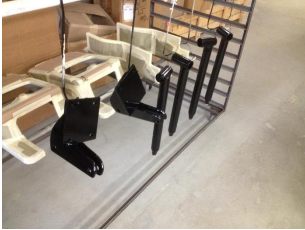
Figure 52 - Axle Mount and Trailing Arms After Powdercoat
