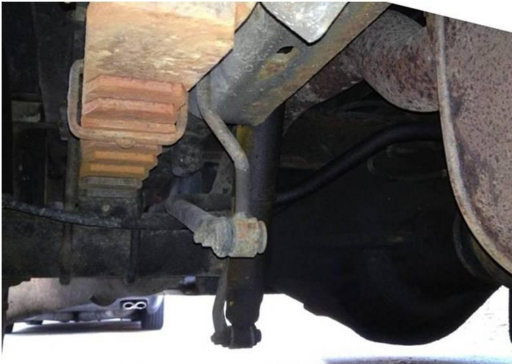
Figure 15 - The suspension setup in our ambulance with the leaf spring (left) and the shock absorber (middle)
