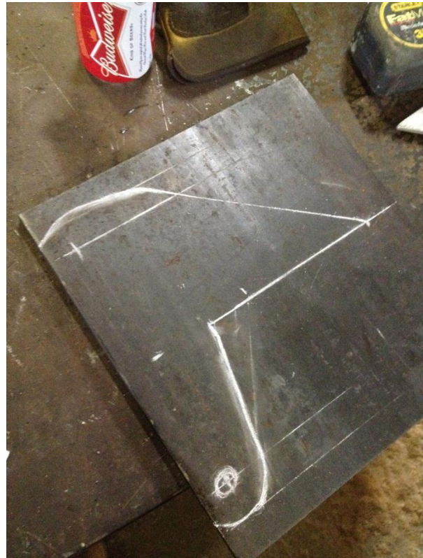
Figure 38 - Axle mount bracket pre-cutout
