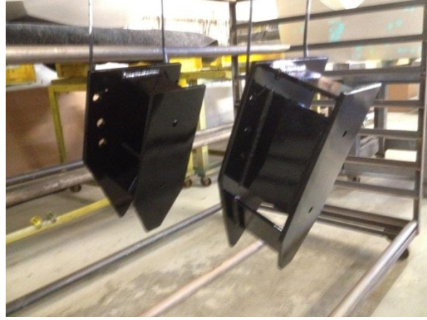
Figure 53 - Front Mounting Brackets After Powdercoat
