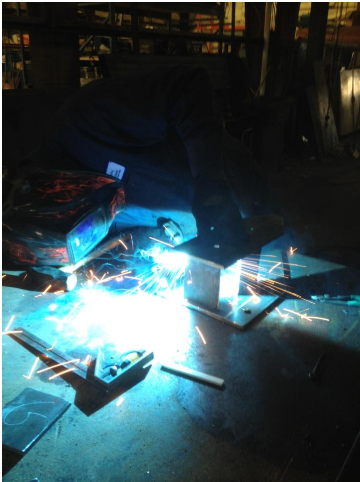
Figure 44 - Welding front mounting brackets
