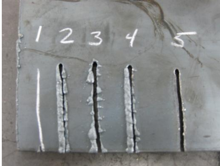
Figure 40 -Plasma cutter cut quality
