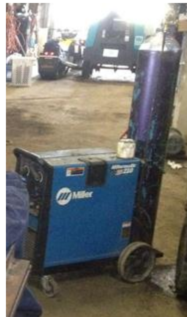
Figure 45 - Miller 220V MIG welder
