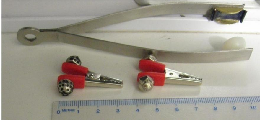
**Figure 5.1. Forceps with cap and track interfaces (top), clip with spherical interface with surface irregularities (bottom left), and clip with smooth spherical interface (bottom right).**
