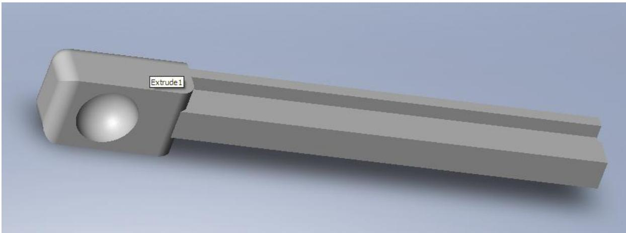
**Figure 12.6. Sliding mechanism that fits into top portion of forceps above**
