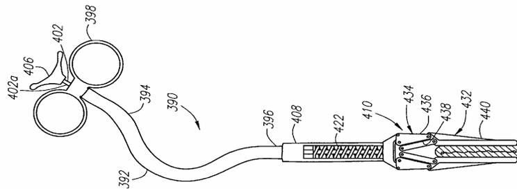
**Figure 2.7. Schematic of flexible clamp applicator (Glines, Morejohn and Septecka 2000)**
