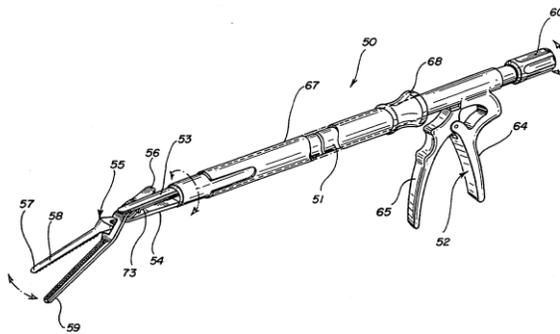
**Figure 2.5. Schematic of endoscopic bulldog clamp (Failla, Hildwein and Lau 1994)**
