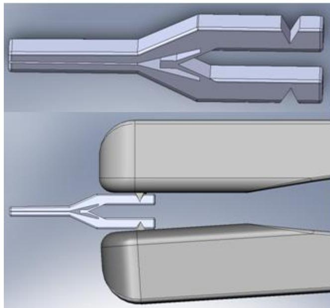
**Figure 2.3. Diagram depicting the groove interface of the currently used clips (top) and the tongue-and-groove interface of the currently used microvascular clip-forceps system (bottom).**
