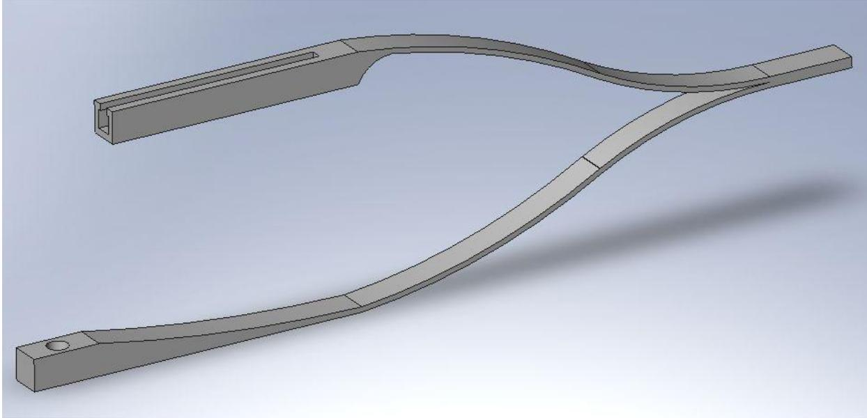
**Figure 12.5. CAD drawing of forceps without sliding mechanism**
