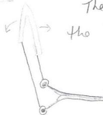
Telescoping forceps with circular end on the tip. The clamps have a cylinder on each end. The circular ends of the forceps slide ~~of~~ over the cylinder to secure the clamp. Since the forceps can telescope they can rotate around the cylinders on the clamp. The forceps can be locked when the desired angle is achieved.
