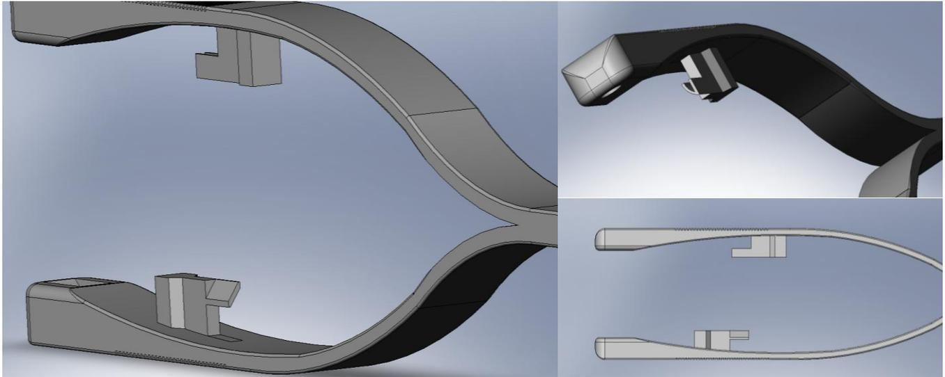
**Figure 9.2. CAD drawing of proposed locking mechanism for forceps device**
