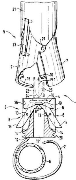
**Figure 2.9. Schematic of a spring loaded clamping device (Matern and Der 1998)**
