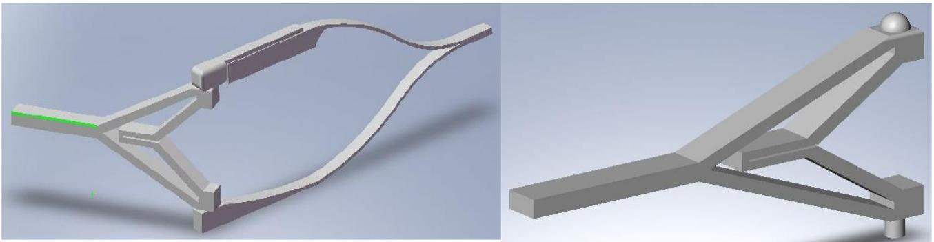
**Figure 4.1. Preliminary design featuring spherical and cylindrical clip interfaces (right) and a sliding mechanism on the forceps (left).**
