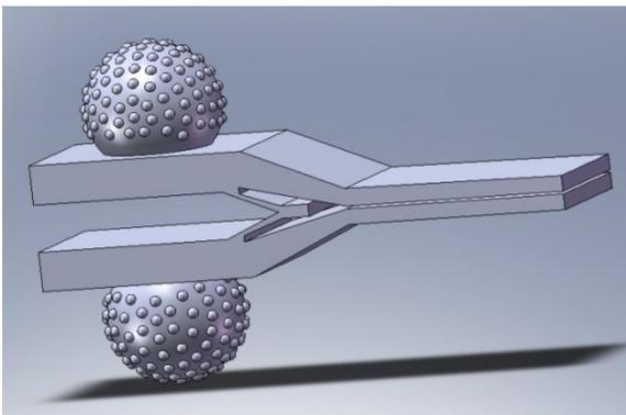
**Figure 12.12.** Spherical interfaces with surface irregularities to allow the clip to be locked into virtually any lateral or vertical angle.
