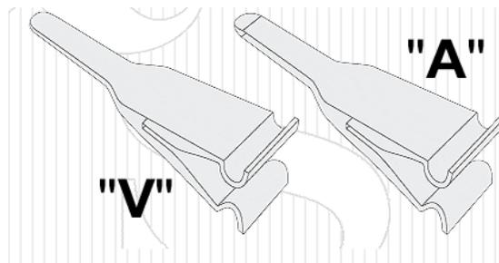
**Figure 12.2. Variations in clamp shape to accommodate for different vessel sizes and pressures (S&T 2007)**
