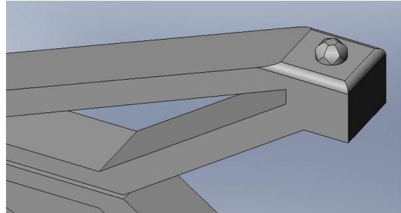
**Figure 12.9.** Hexagonal half-sphere that would function as a ball-end hex key to lock the clamp into different angles.
