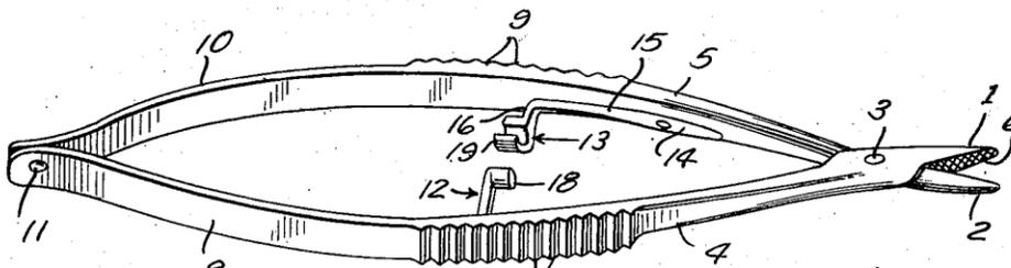
Figure 9.1 Schematic of Castroviejo Locking Mechanism (Castroviejo 1953)
