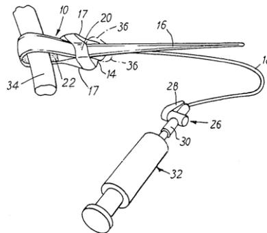
**Figure 2.8. Schematic of inflatable tube application (Dunn and Scarrow 1985)**
