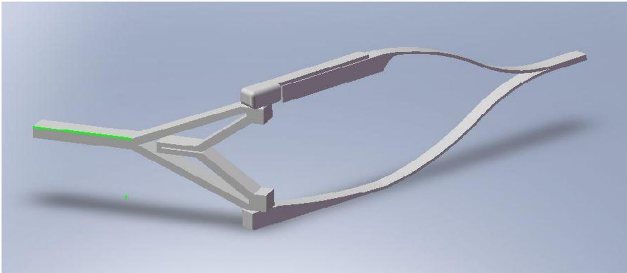
Figure 12.3. This image depicts the full assembly of the initial forceps, sliding mechanism, and clamp design.
