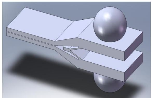
**Figure 12.11.** Smooth spherical interfaces that would allow unlimited vertical and lateral rotation based on friction.
