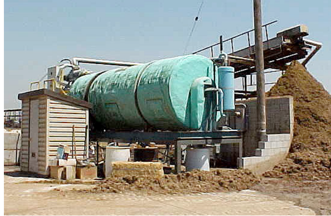
Figure 7: Typical In-Vessel Composting System (EPTCorp, 2004)
