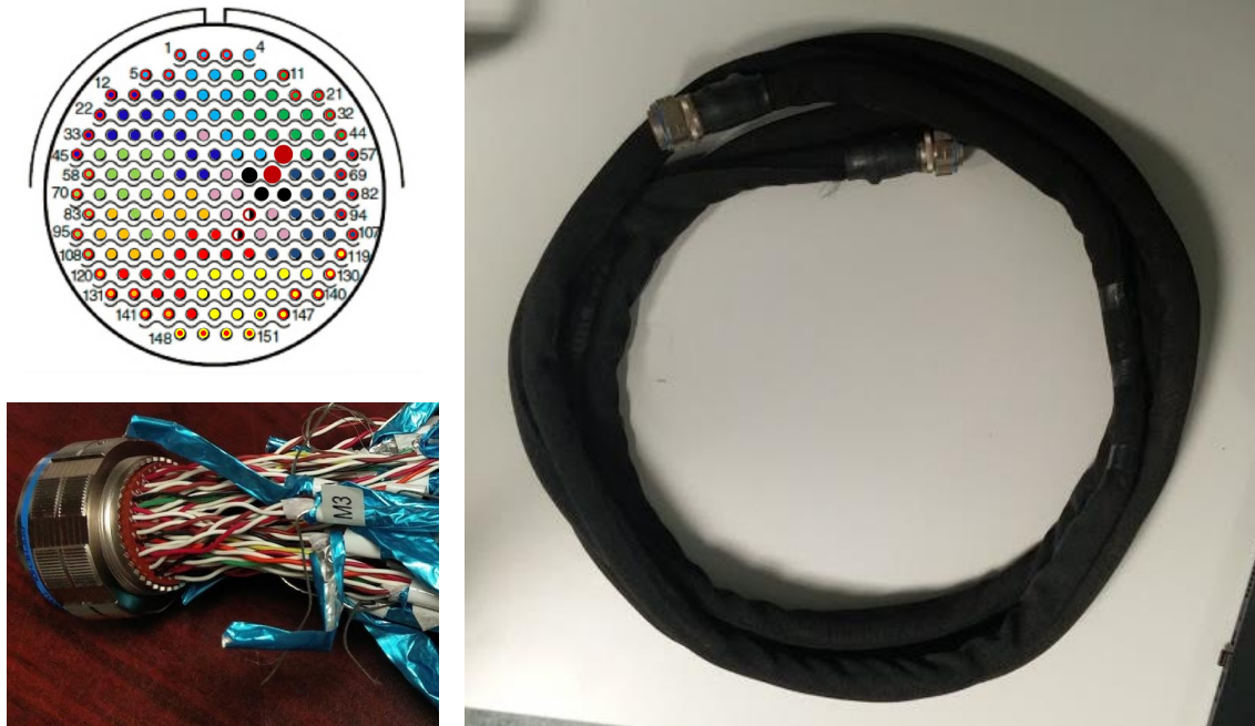
Figure 5.7: Custom cable design: left showing layout of 151 conductors color coded pin-out to identify each encoder and motor power cable clusters and on the right showing the final assembled cable
