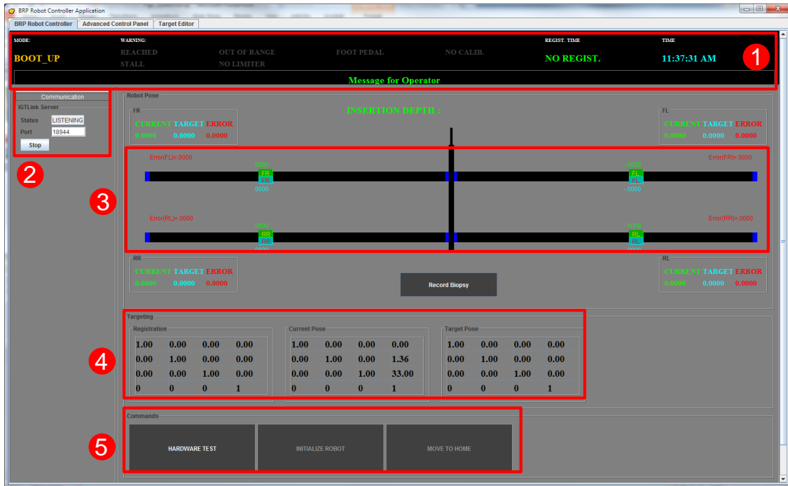
Figure 2.8: Clinical robot control application (CUI) showing: (1) robot status information, (2) OpenIGTLink connection status with the navigation application, (3) current and target robot joint positions, (4) robot pose, registration transform and target transform and (5) control buttons for robot hardware test and initialization.
