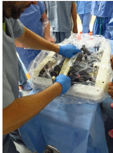
Figure 0.14 Drape the robot and push the front piece in
