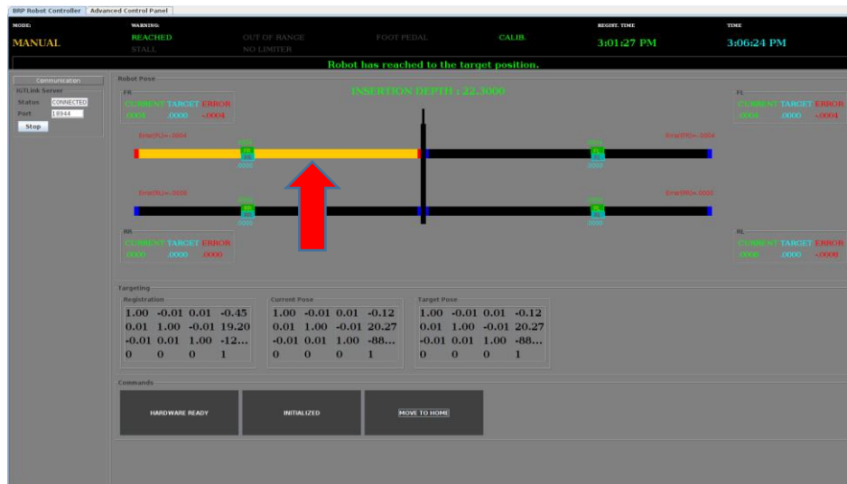
Figure 9.3 Indication of Limit Switch Error ( Orange link bar with limit indicators turned to Red )
