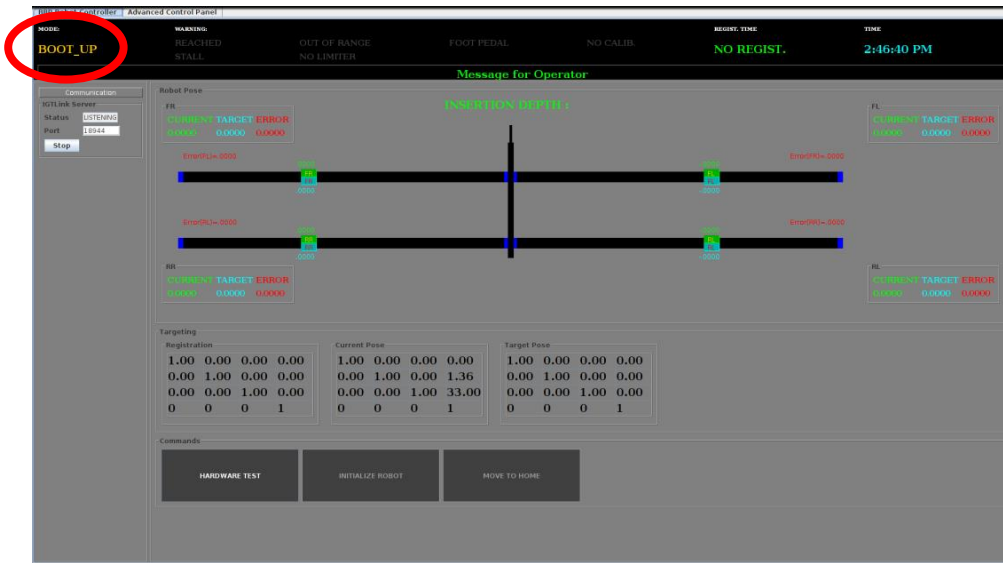
Figure 3.3 BOOT_UP mode, homing procedure is not yet executed
