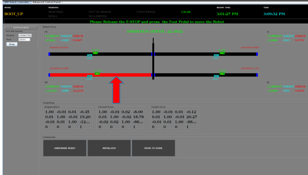
Figure 9.8 Indication of Stall Switch Error (Red link bar)
