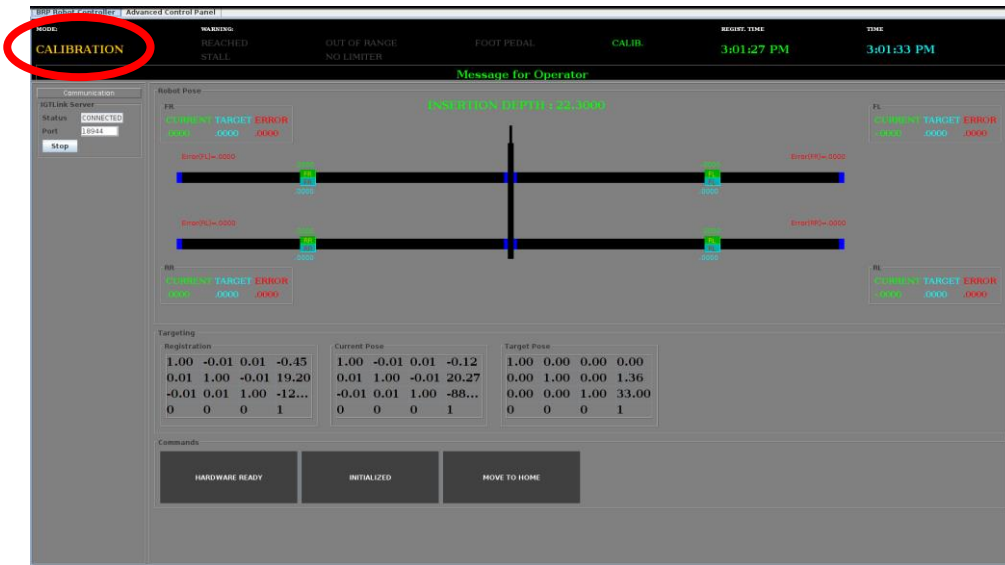
Figure 7.4 Robot Control application after receiving valid CALIBRATION transform
