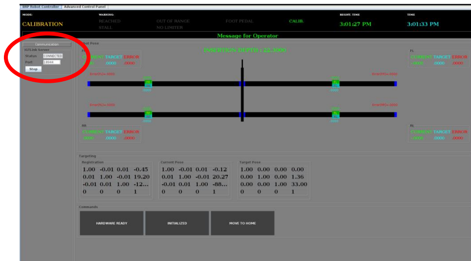
Figure 4.6 IGTLServer status changed to CONNECTED on RadVision connection
