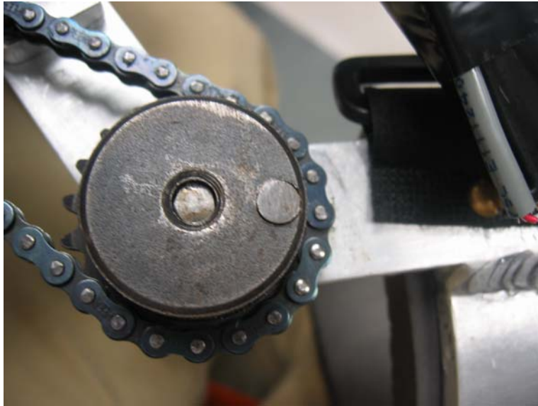
Figure 48: Elbow Gear and Forearm Cage of Proof-of Concept Prototype
