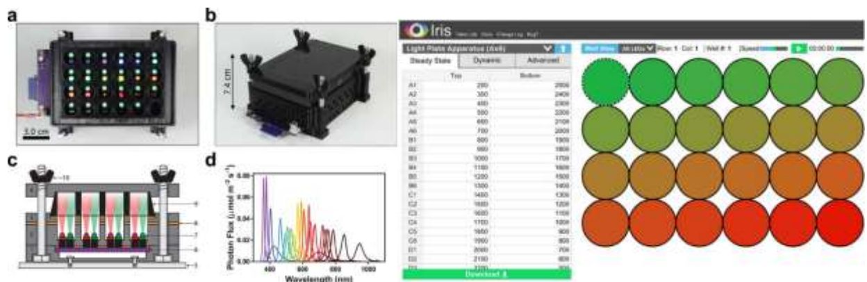
Figure 2: Model of the Light Plate Apparatus (left) and digital view of the LPA programming platform IRIS as proposed by Dr. Jeff Tabor’s laboratory at Rice University. 27
