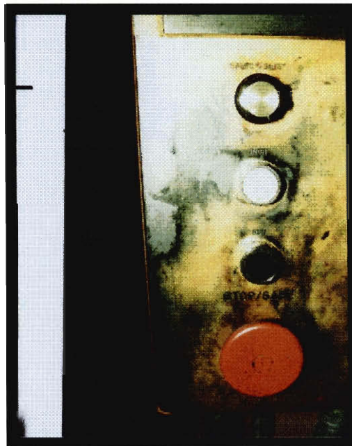
(picture of control unit containing speed adjust, inch button, start button, and stop button from top to bottom)
