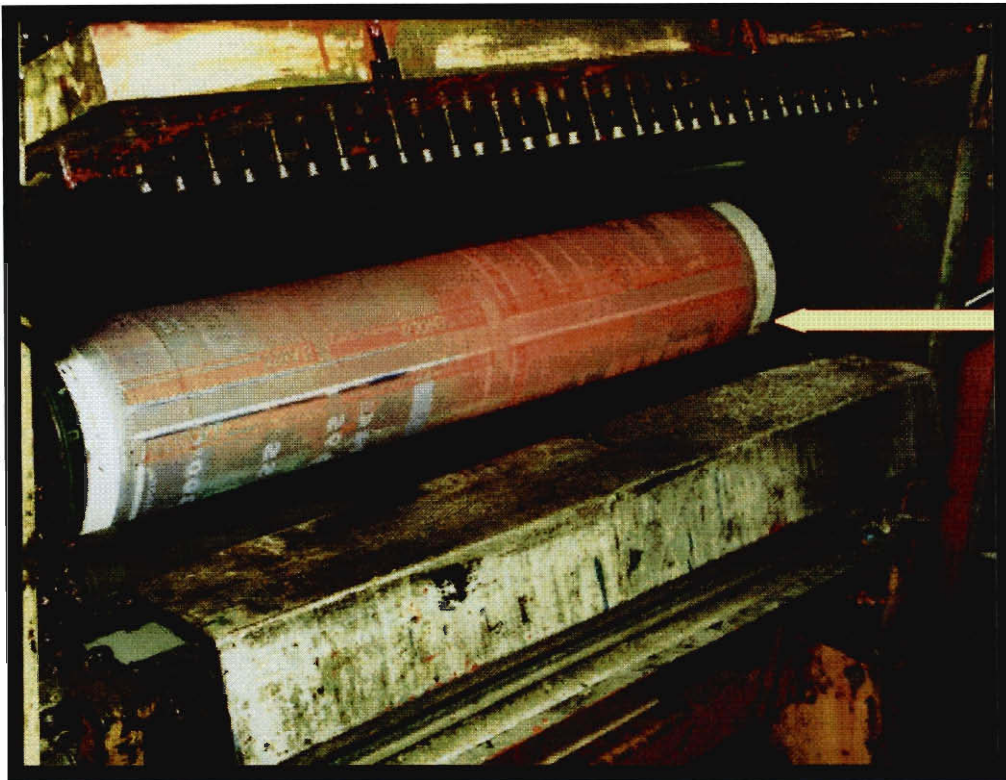
(A picture of the press without the guard, the yellow arrow points to an exposed nip point)
