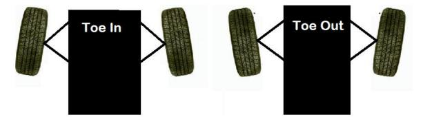
Figure 18: Toe-In and Toe-Out
