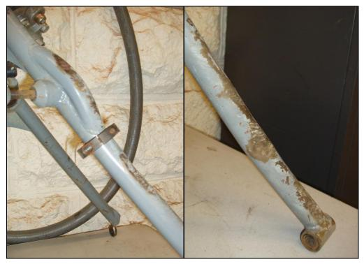
Figure 34: Damage to Left and Right Lower Control Arms
