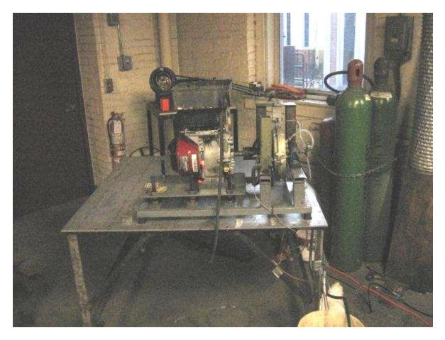
Figure 2: Engine Dynamometer Test Stand
