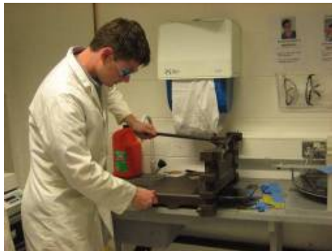
Figure A7-2: Cutting PCB board to size
