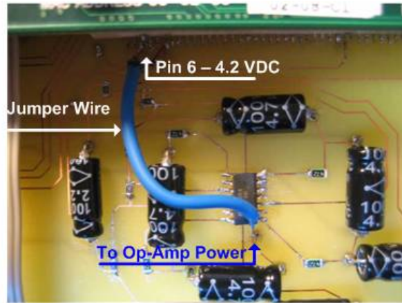
Figure 7-23: Temporary Solution for LP324M
