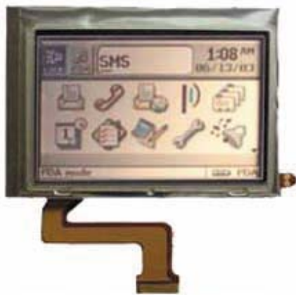
Figure 5-6: Front view of the Sony ACX075AKM-7.
