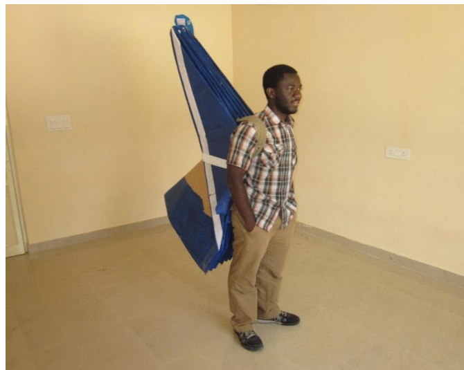
Figure 14. Full scale dome prototype in compressed form.
