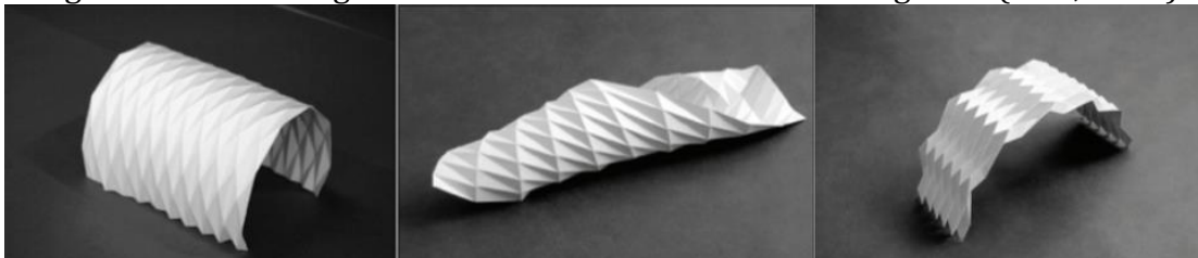
Figure 4. Diamond, Diagonal, and Herringbone folding patterns seen from left to right.
