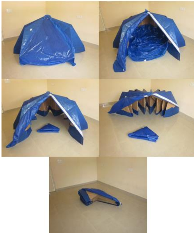
Figure 15. Shelter transforming from popped up to compressed.
