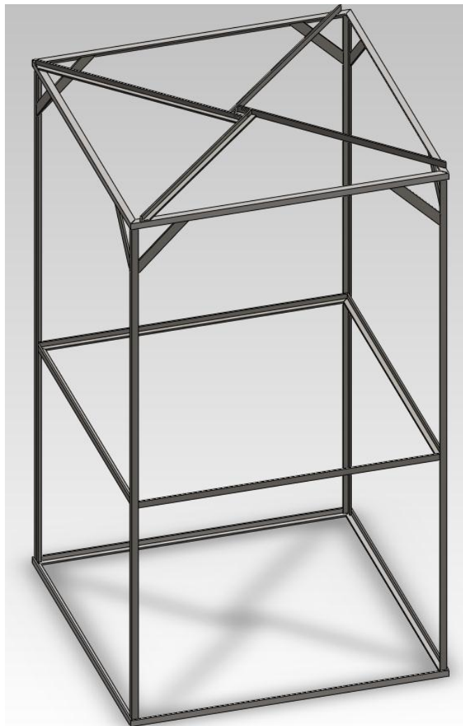
Figure 18 - Final Support Frame Design
