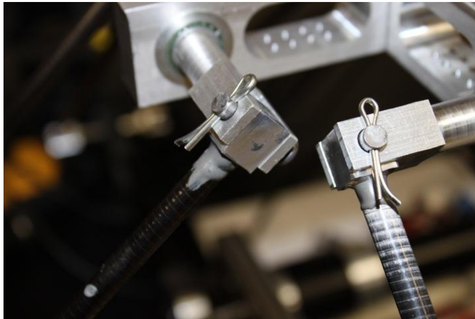
Figure 12 - Final U-joint Assembly
