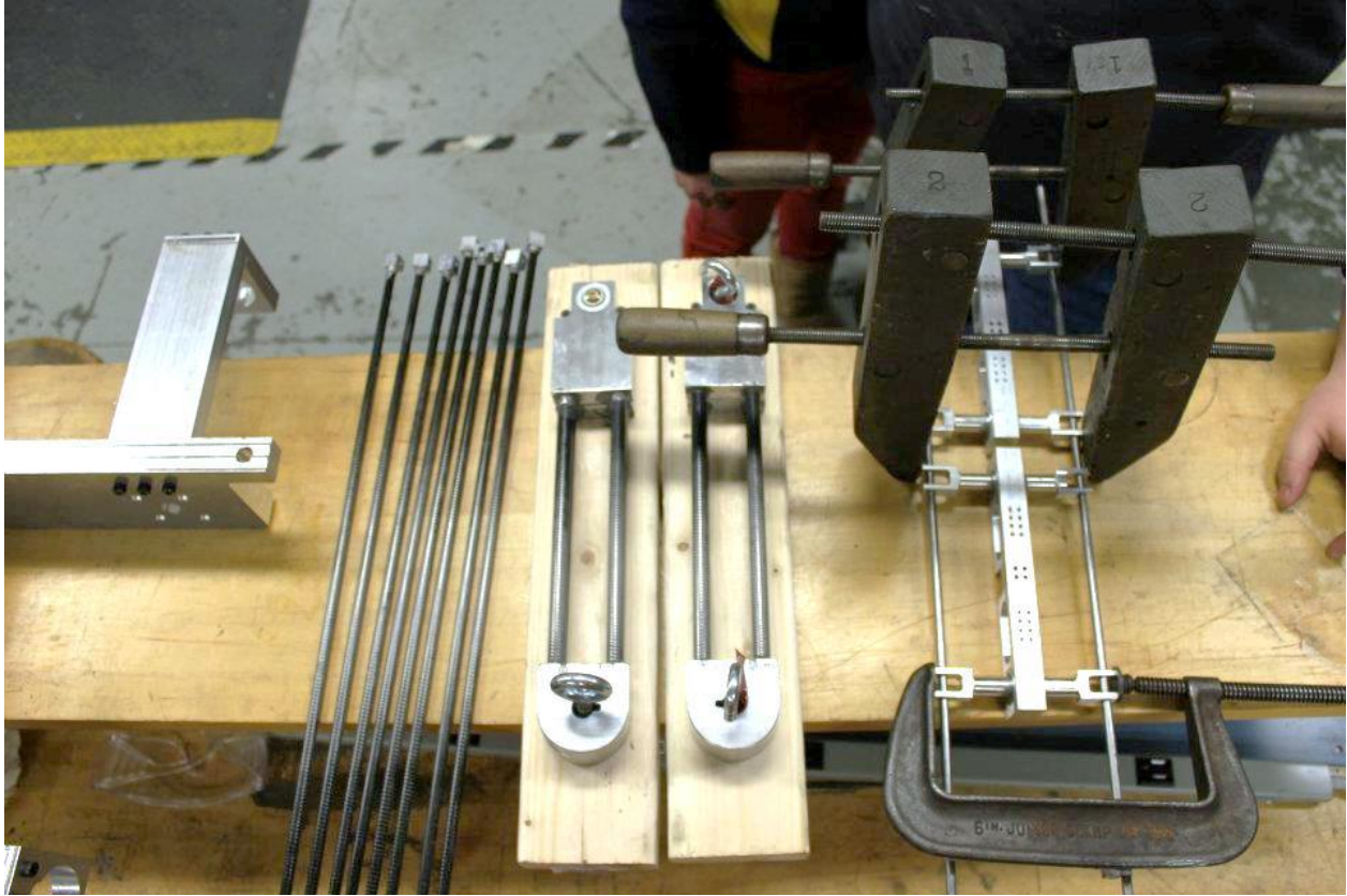
Figure 14- Subassemblies during epoxy setting
