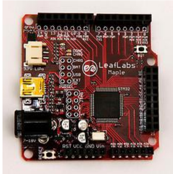
Figure 20 - The Maple LeafLabs Board based on ARM Cortex-M3 Architecture
