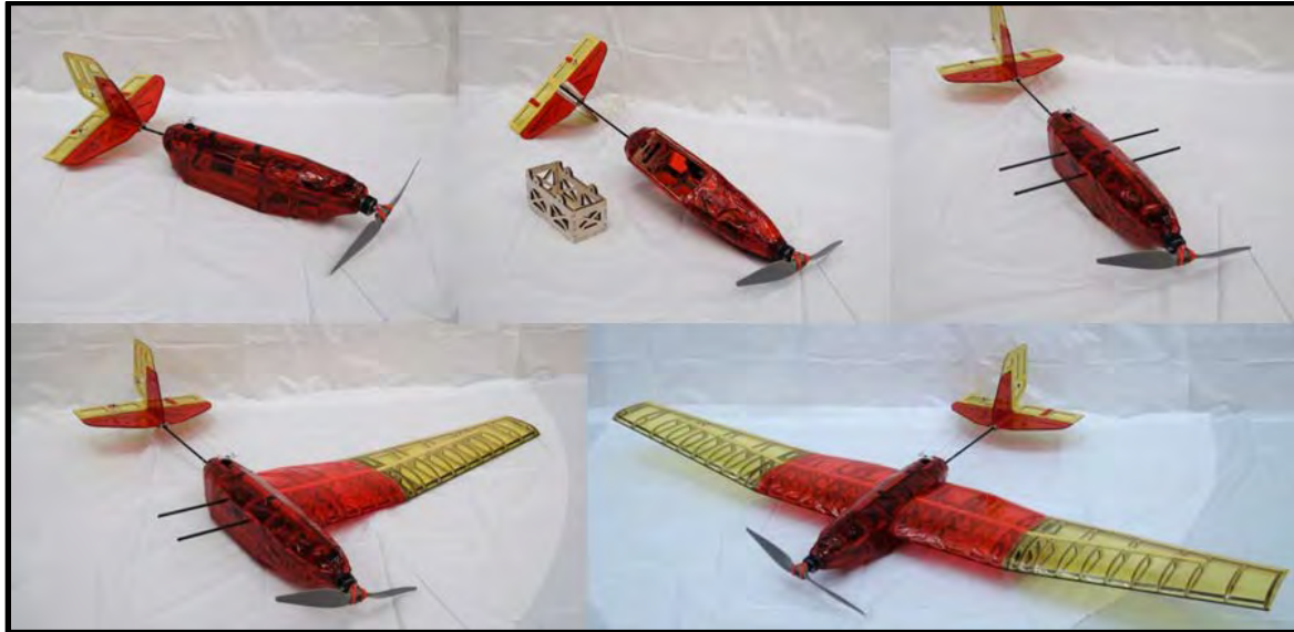
Figure 15: Final Assembly Montage
