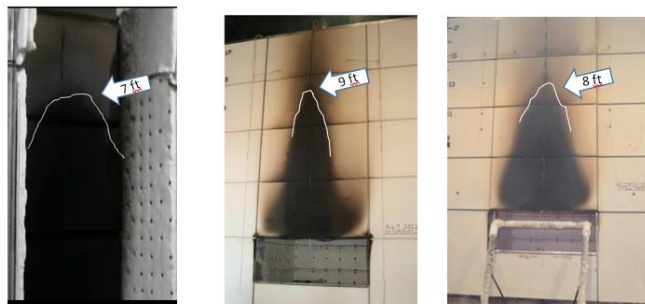
Figure 6: Left to Right, Final burn pattern of last year’s experiment. The white line is drawn to distinctly show the char pattern, Final burn pattern of Southwest 1, Final burn pattern of Southwest 2
