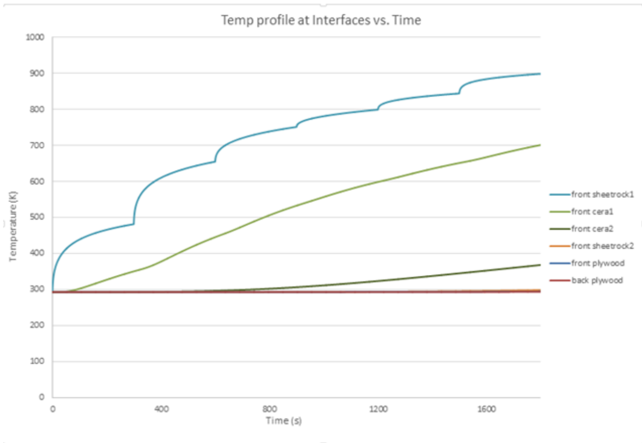
Figure 69: Temperature profiles at 5min intervals with 2 layers of cerablanket
