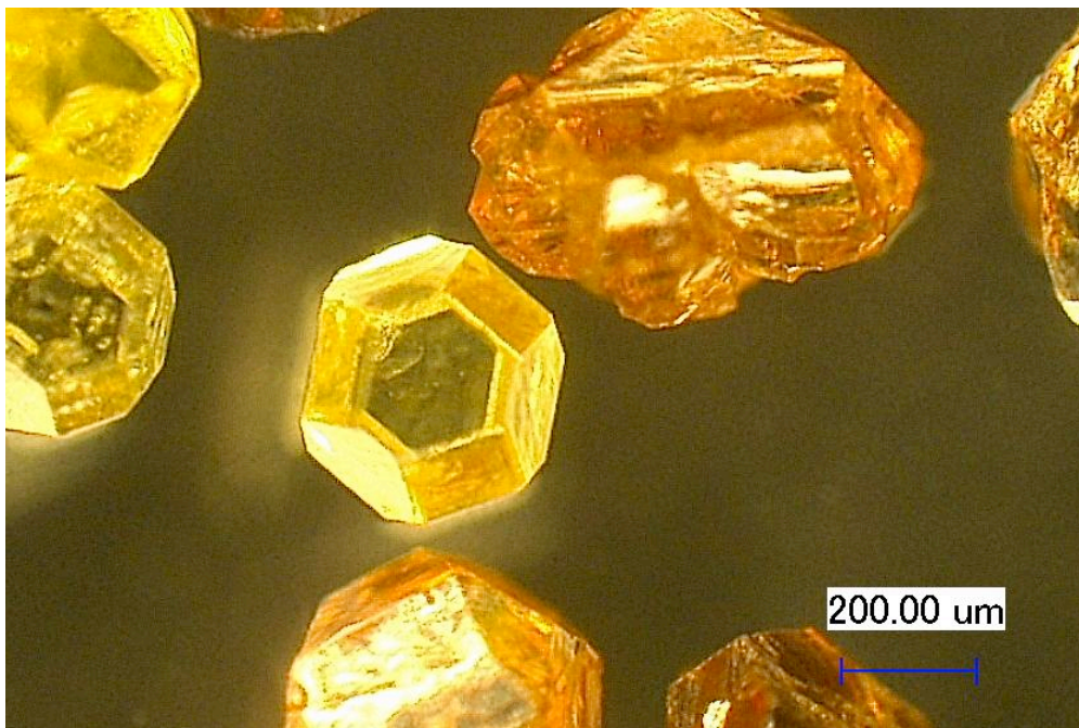
Figure 5 - CBN Grain Under High-Powered Microscope
