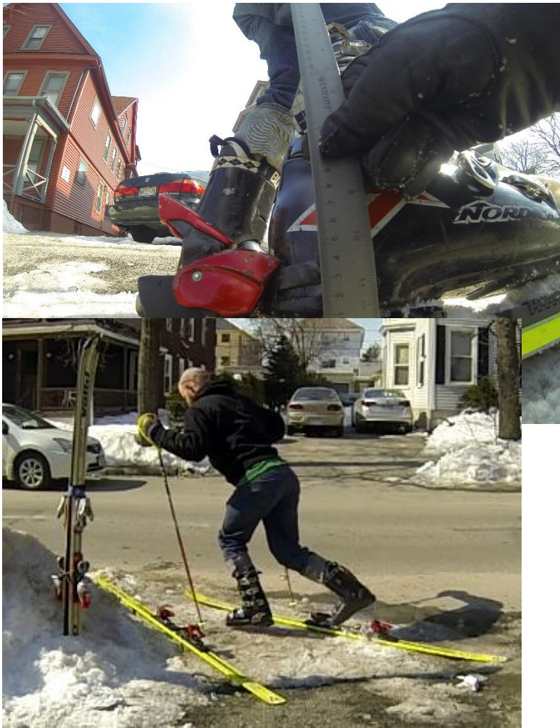
Figure 15: (both heel and toe units of the ski binding are packed with roughly a \frac{1}{4} " of compacted ice.)
