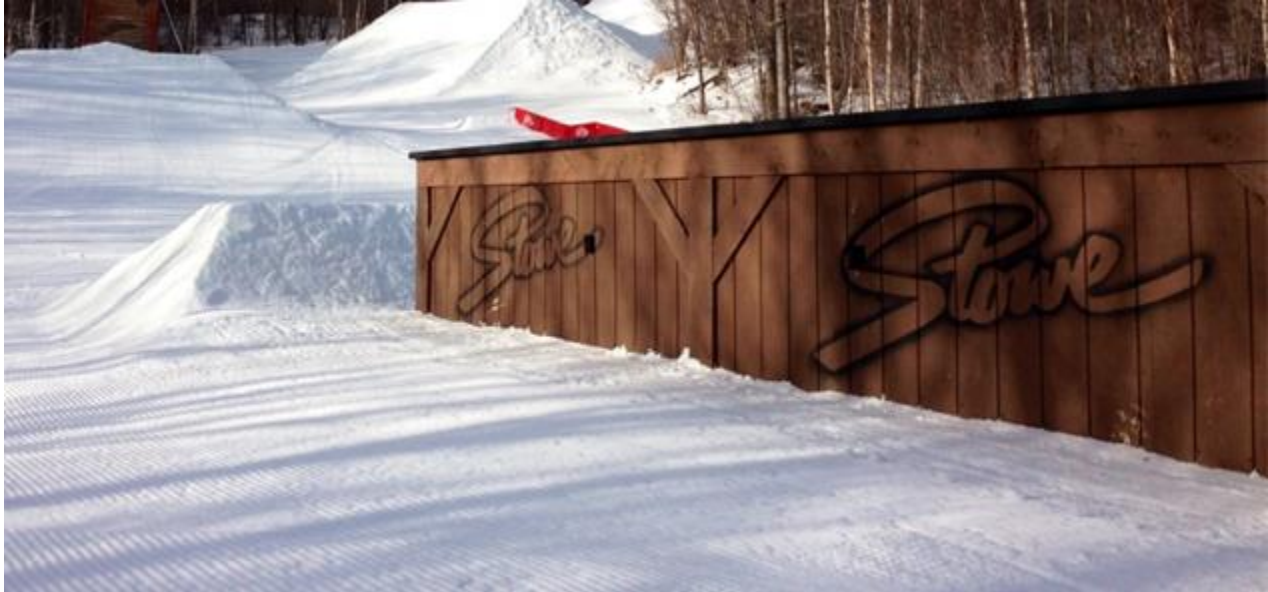
Figure 9: Mt. Stowe Box. This box is a wooden structure with an 8-inch flat metal surface. This allows the rider to balance his or herself better due to the larger surface area. The height of the box is 4 feet tall and it is thirteen feet long. This is one of two boxes that are in the terrain park. The other box was much smaller in size and easier to attempt.
