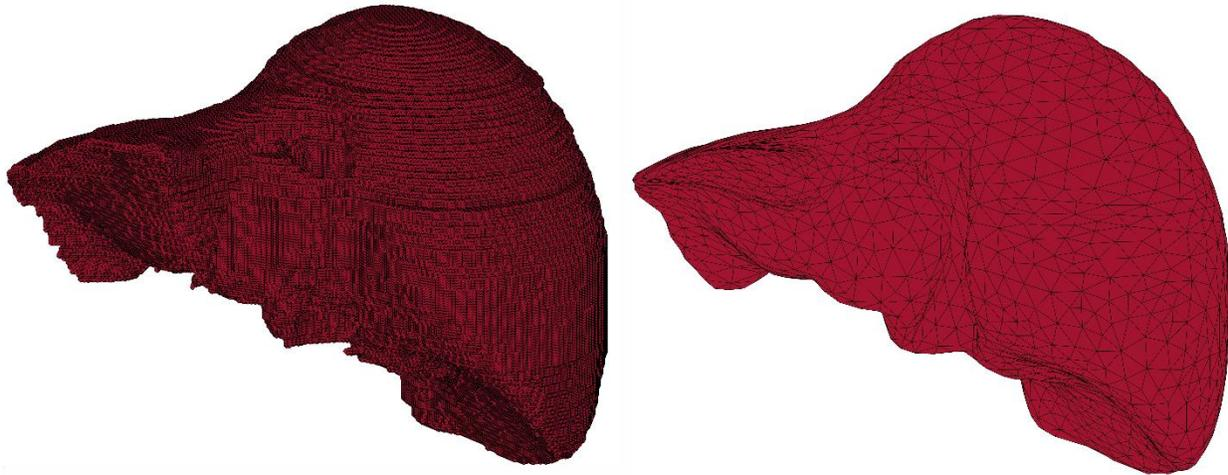
*Figure 4: Liver Voxel Model (Left) and Liver CAD Model (Right)*
