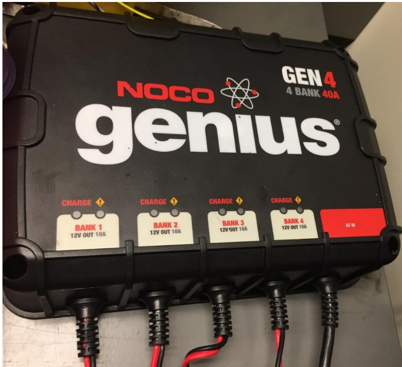
Figure 63: NOCO genius GEN4 battery charger that was used on the Goat Cart and was replaced by the 2017-18 team. It had automatic shut-off, but it is not a float charger. [33]
