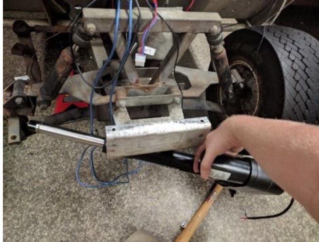
Figure 28: possible mounting of linear actuator in front of the Cart's suspension. This would not require the removal of the original steering rack.
