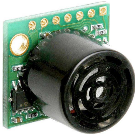
Figure 73: The LV-MaxSonar-EZ3 ultrasonic sensor module used in the ultrasonic system. This sensor module is a narrow beam ultrasonic sensor with good side object rejection, low power consumption, easy to use interface, large object detection and can be powered by many different types of power sources [9].
