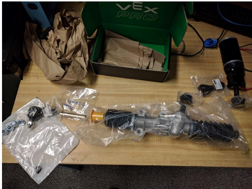
Figure 29: Lay out of the new steering components on table prior to installation.
