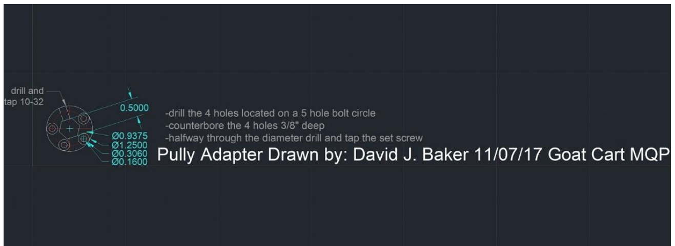
Figure 30: Pulley Adapter CAD Drawing
