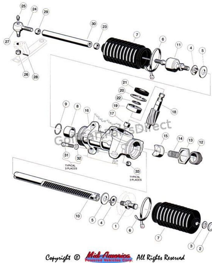
Figure 22: Explosion of the steering rack system in a 1995 Club Car DS [22]
