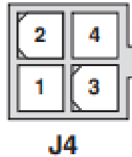
Figure 60: Diagnostic pin cluster diagram for use with programmer or external LED. Table 10 elaborates on the different pinouts. [31]
