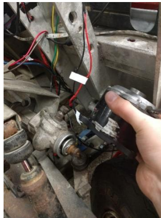
Figure 26: Possible mounting location if the motor is used to drive the original steering rack of the can
