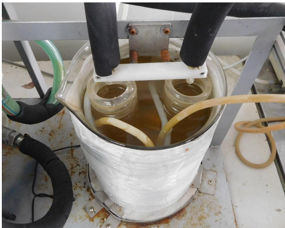
Figure A6: Vessel containing the cooling water in which permeate stream flows through in the two coiled tubes.
