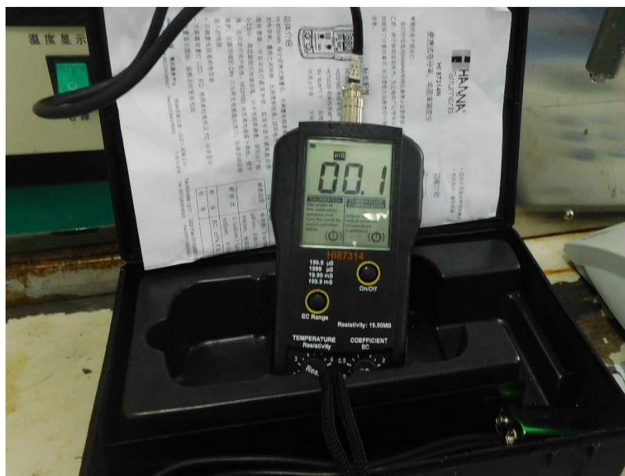
Figure A10: Black conductivity meter used for the first two weeks to measure feed solution conductivity and the final five weeks measuring feed and permeate solution conductivity.
