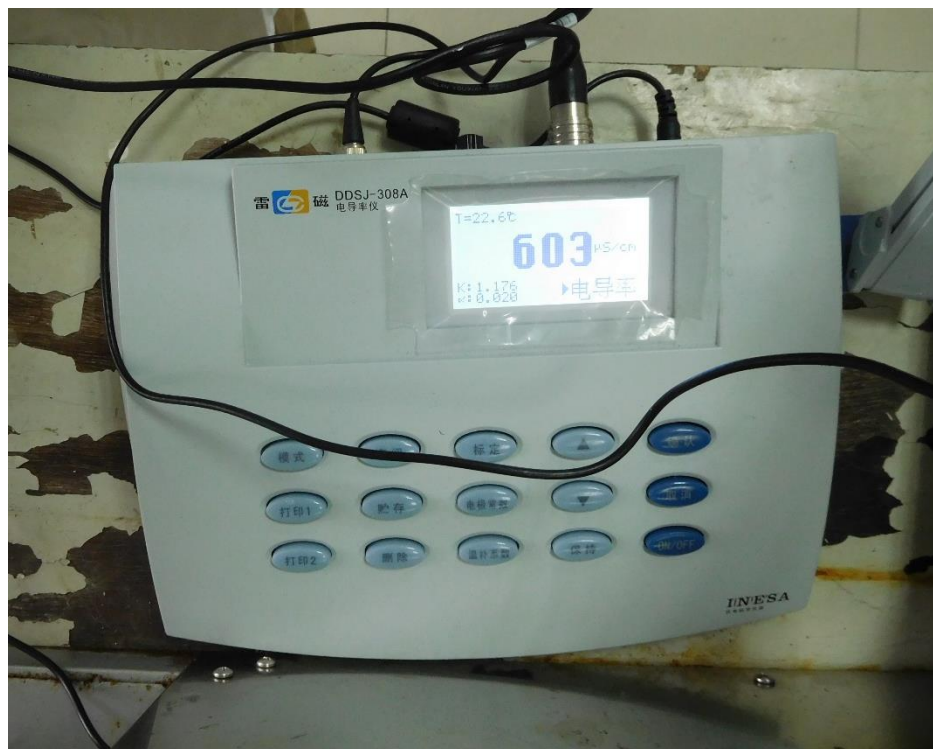
Figure A11: White conductivity meter, used to measure the conductivity of the permeate solution for the first two weeks of testing.
