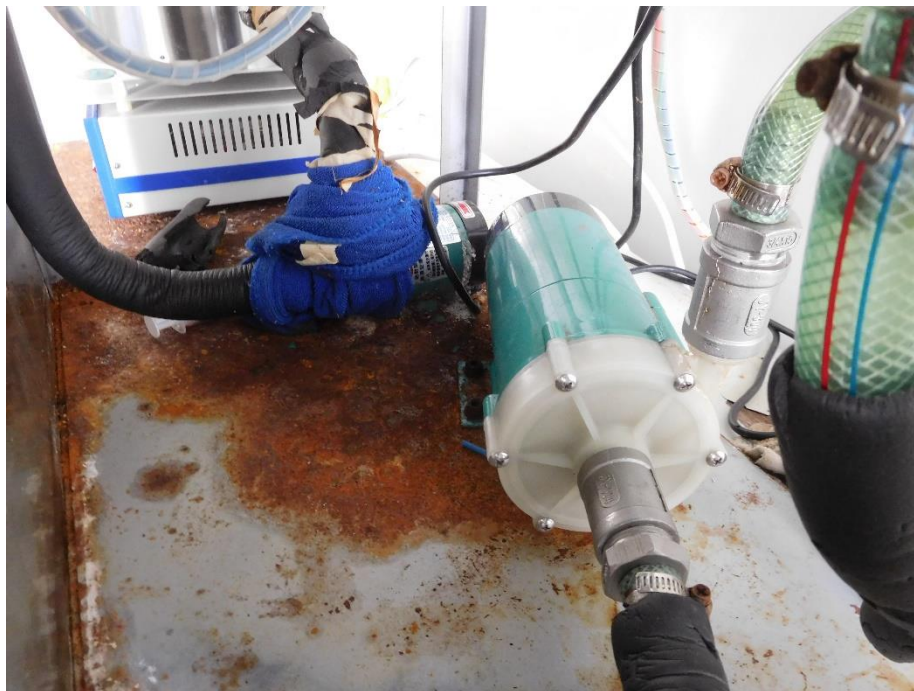
Figure A13: Two pumps used in distillation process; small pump for feed, large pump for permeate.
