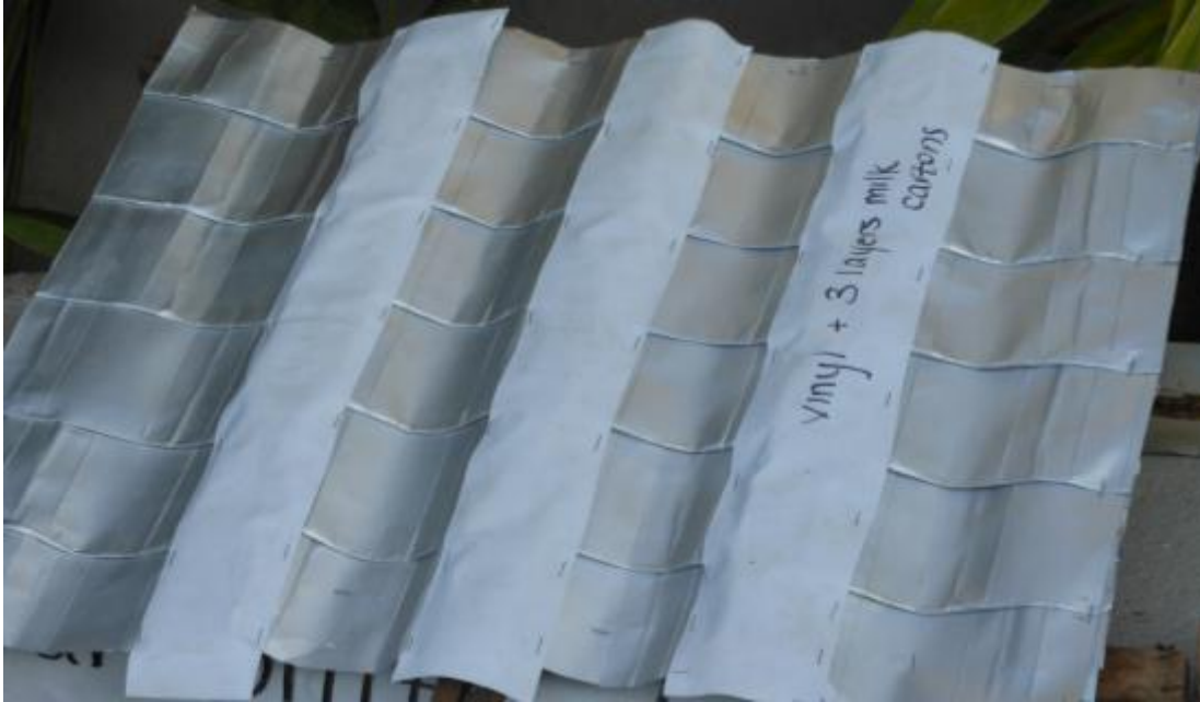
FIGURE 16: HYBRID TETRA PAK WITH VINYL SOLUTION
